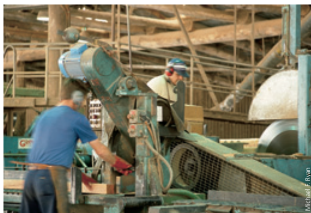
Docking sawn timber
