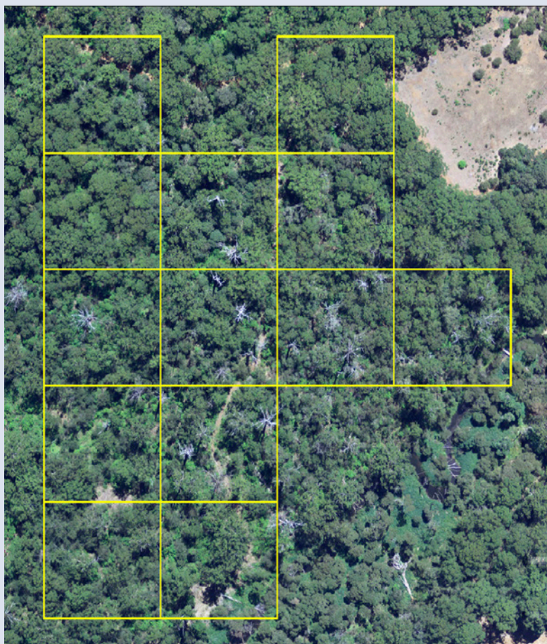
Figure 1.15: A systematic grid of cell size 0.5 hectare used to record the occurrence of stumps, landings, snig tracks and other disturbance features for the assessment of old-growth forest status in karri forest near Pemberton, Western Australia
