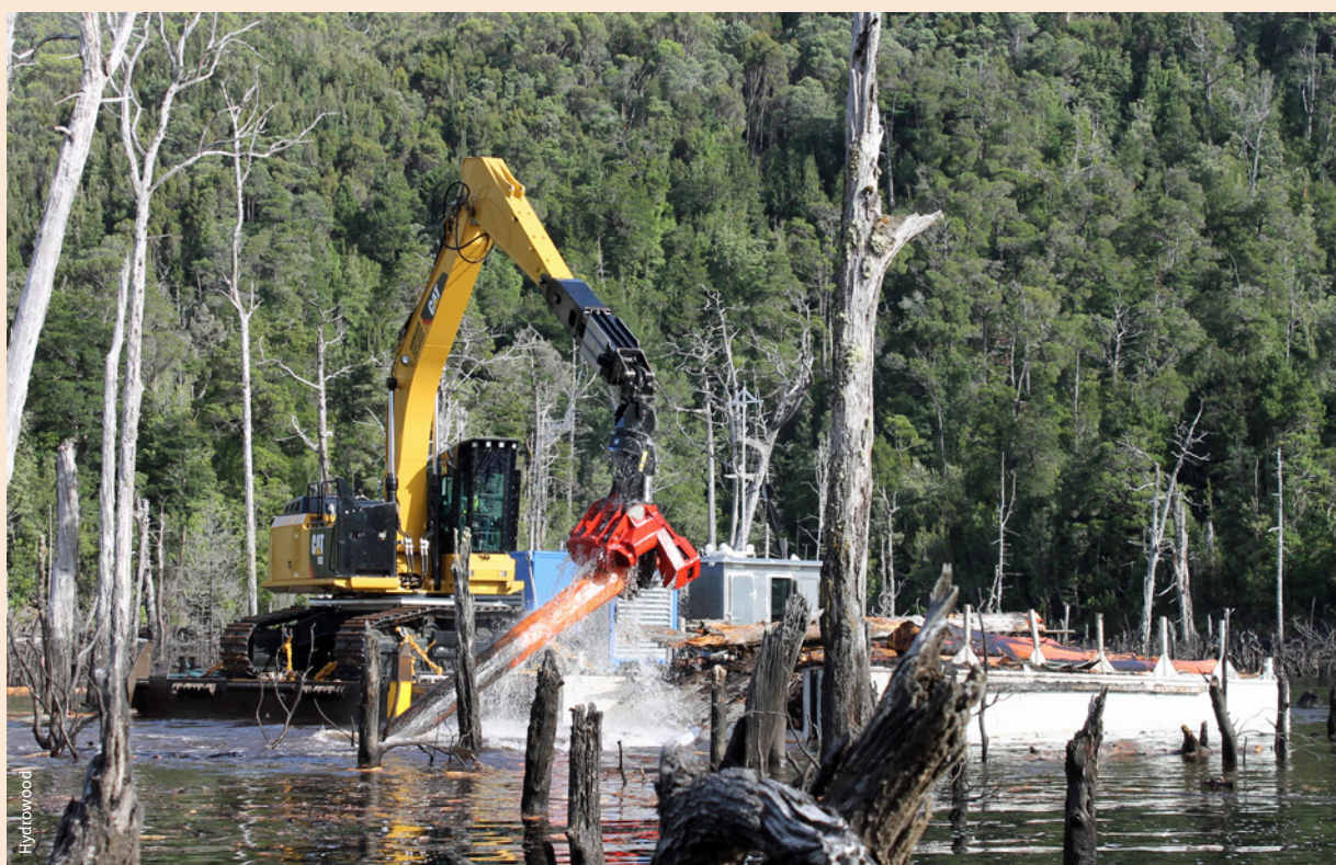
Hydrowood purpose-built, waterproof harvesting head and boom attached to an excavator mounted on a barge.
