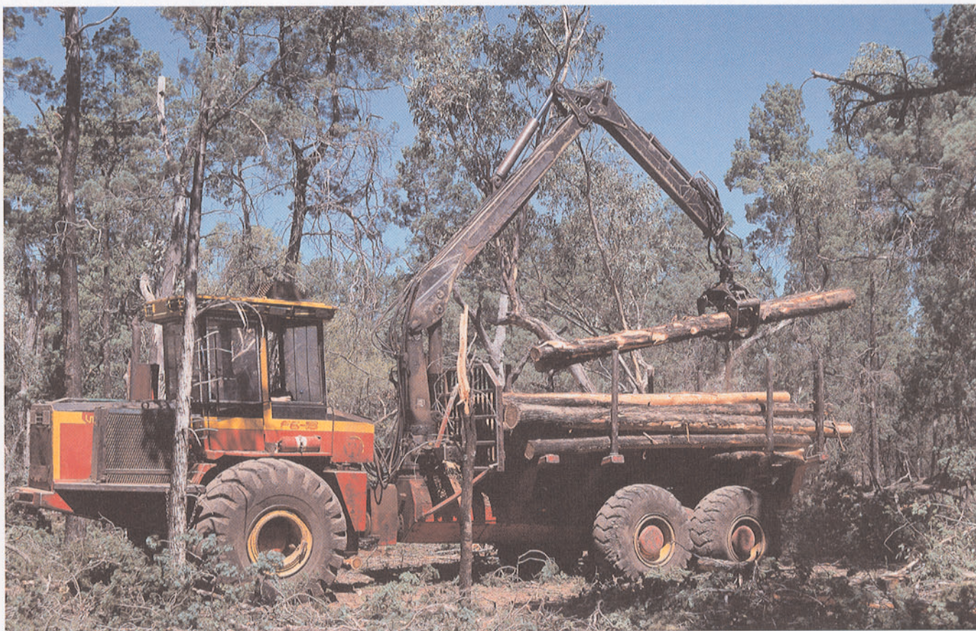
Forwarder collecting white cypress pine sawlogs that have been felled and delimbed (New South Wales).
