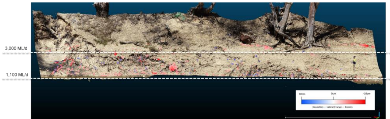
Figure 12-4 DEMOD illustrating change in response to Spring Fresh event at McCoy's Bridge bank C.
