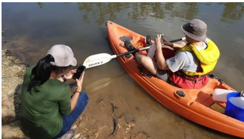
Figure 7 Connecting HOBO loggers via Bluetooth to a smartphone to take light and temperature measurements.
