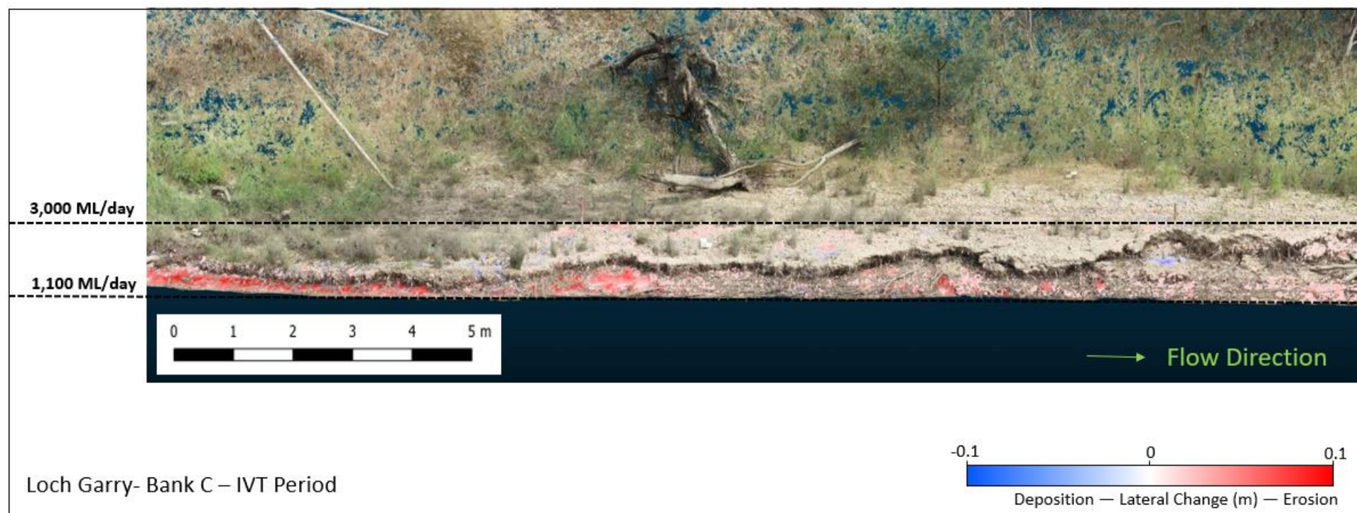
Figure B-5 DEMOD illustrating change in response to IVT period at Loch Garry bank C.
