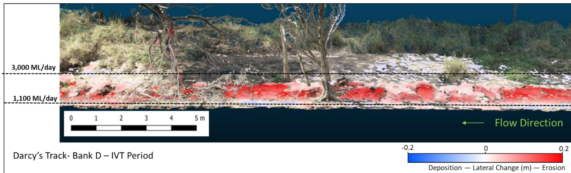
Figure B-4 DEMOD illustrating change in response to IVT period at Darcy's Track bank D. Note the wider colour scale (-0.2m to 0.2m) to capture the large magnitude changes.
