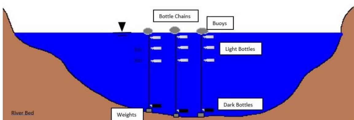
Figure 6 Diagram of the bottle chains setup in the river
