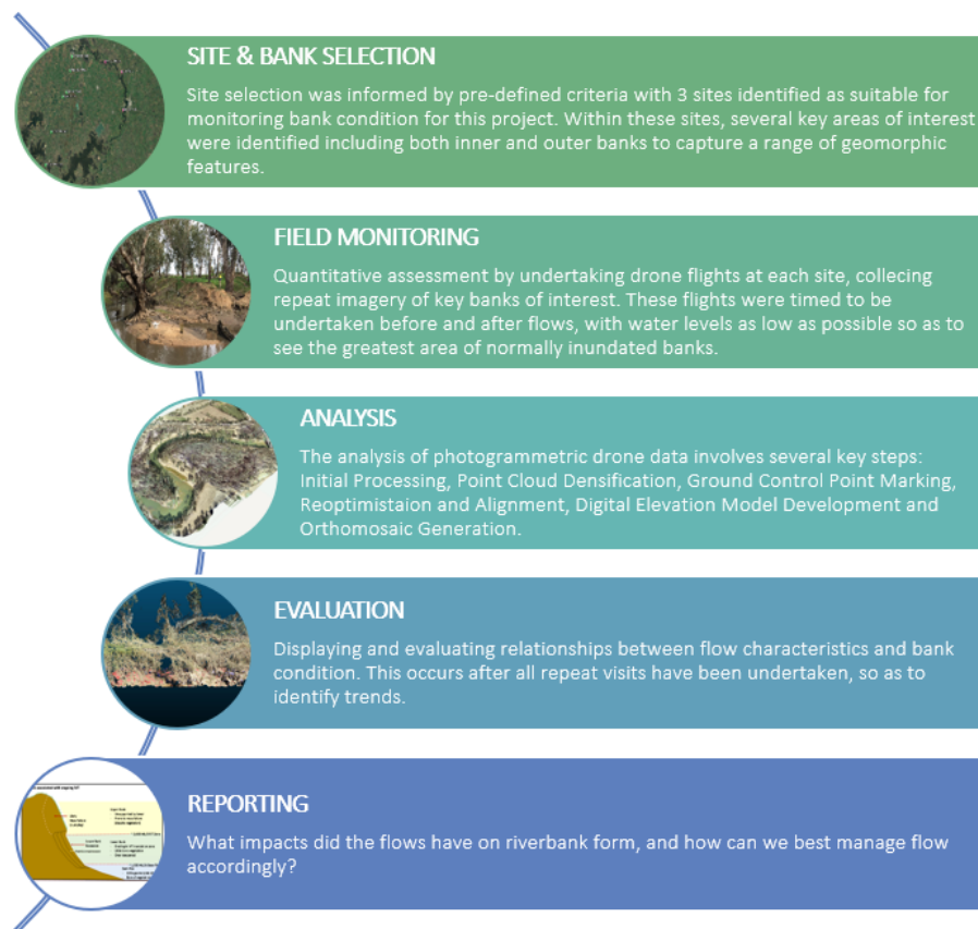
Figure 4-4 Infographic providing an over-view of the methodology applied to bank and vegetation condition analysis using UAV technology (Streamology & Arthur Rylah Institute 2020).
