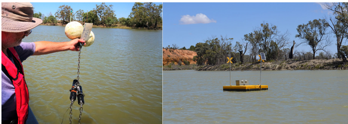
Figure 6. Loggers that are deployed in the Lower Murray River to measure dissolved oxygen concentrations (left) and the typical mooring station (right) (photos: SARDI).
