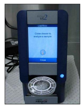
**Figure 3.** The compact in-house VetScan VS2<sup>TM</sup> Chemistry Analyser installed and running in the laboratory at James Cook University. The blood sample is loaded into the rotor and then the rotor is placed in the drawer. Sample analysis takes approximately 8 minutes, at the end of which a print out listing the values for 12 individual analytes is produced. Photo by S. Young.
