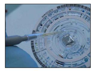
**Figure 4.** Loading a blood serum sample into the VetScan VS2<sup>TM</sup> Chemistry Analyser rotor. Note the extremely small sample size required (100 microlitres, or 0.1 ml), allowing the full panel of analytes to be run even with the small sample volumes collected from frogs. Photo by S. Young.
