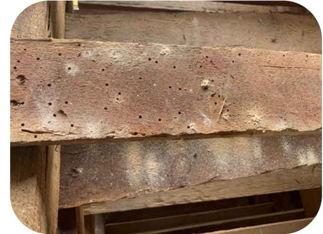
Borer holes with frass in timber packaging.
