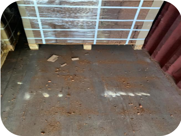
Frass visible on floor once timber pallets removed. A clear indicator of active borers.
