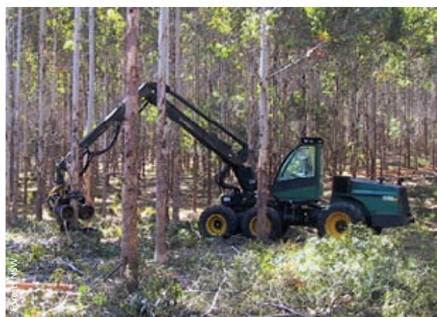
Depending on soil type and weather conditions, the choice of machinery, wheeled (above) or tracked (below) may determine the intensity of impact on soils during harvesting.
