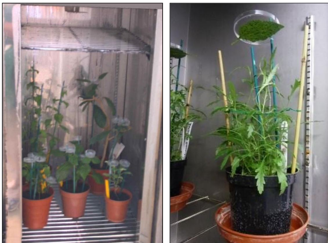
Figure 9. Dew chamber used for rust infection in all experiments. (left) qualitative method of inoculation of host test plants; (right) quantitative assessment of susceptibility of Verbena gaudichaudii .
