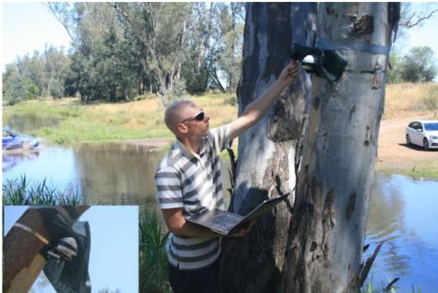
*Figure 7: Setting up a dendrometer band and logger for measuring changes in tree stem diameter over diel and seasonal time periods. Inset shows detail of dendrometer and logger. The species is *Eucalyptus camaldulensis* situated at the perennial riparian site at Maules Creek.*
