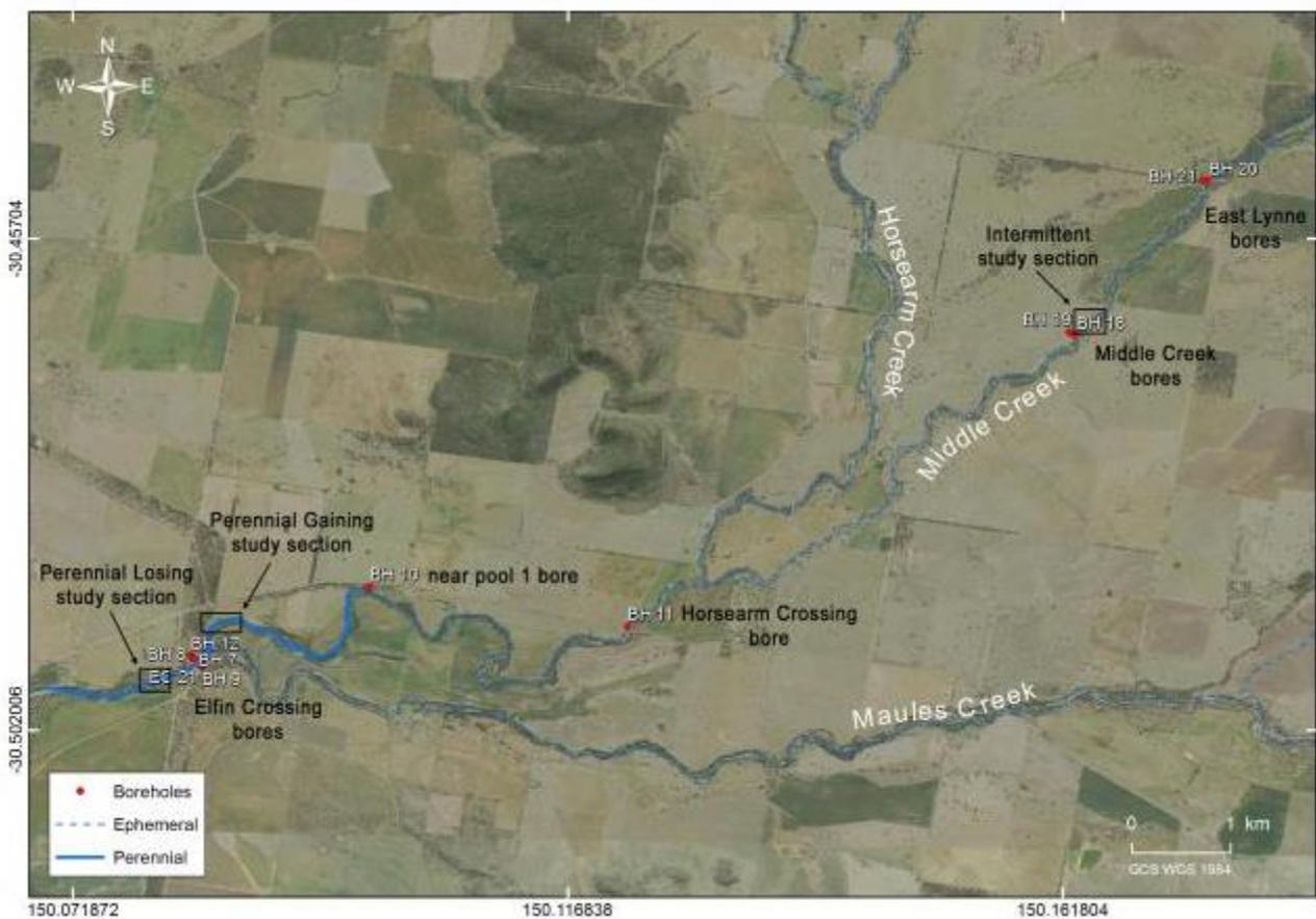
Figure 65: Maules Creek catchment study area indicating base-flow regimes in Maules Creek, Horsearm Creek and Middle Creek, and showing bore infrastructure.
