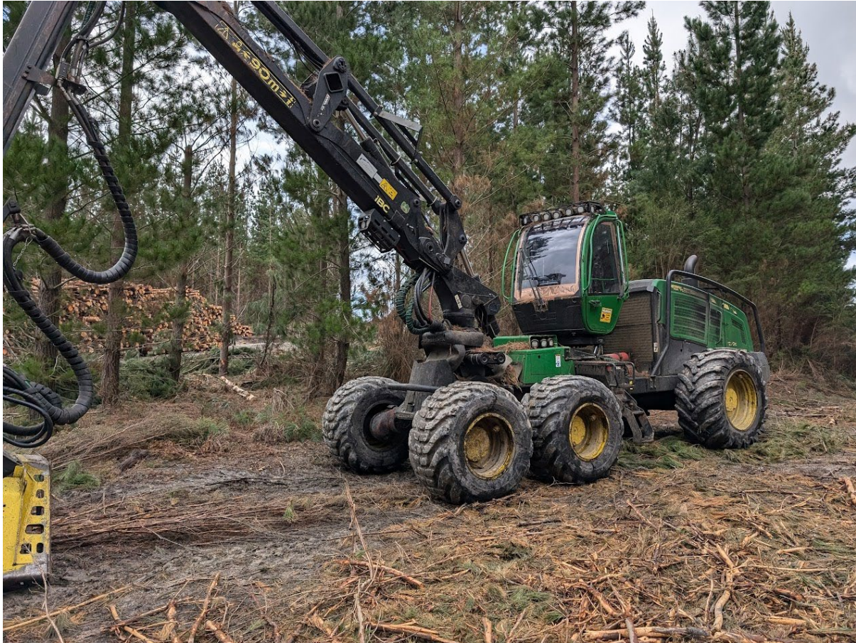
Figure 3: Plantation harvesting in Gippsland, with slash protection of soils
