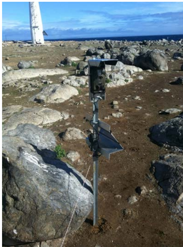
Figure 9. A remote camera deployed on Dangerous Reef, Spencer Gulf, South Australia. This system uses a motion activated camera and photos are stored on removable memory and/or transmitted via the mobile telephone network. Power is provided by a small solar panel. Photo by Mark Whelan, from Goldsworthy et al. (2013).
