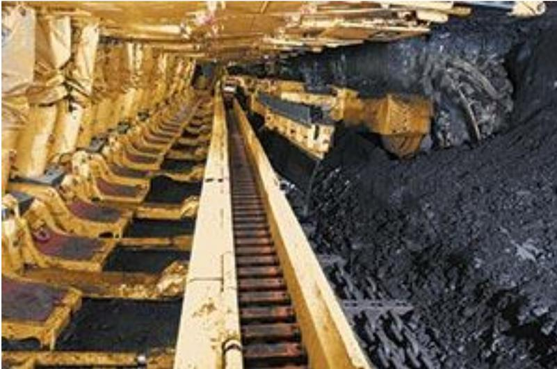
Figure 4 Typical shearer, conveyor and hydraulic support chocks (© Copyright, Caterpillar 2013).
