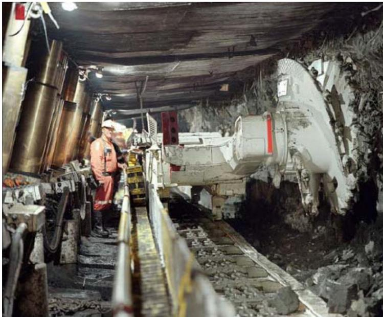
Figure 1 An operating longwall face (© Copyright, MSEC 2007).
