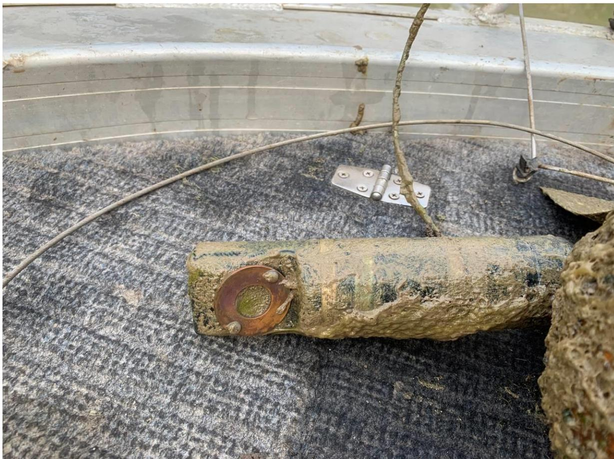
**Figure 16: Algal growth on dissolved oxygen sensor at Collarenebri weir pool**
