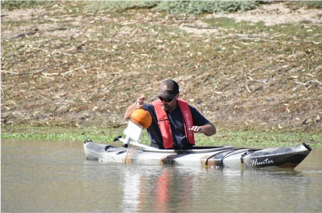
**Figure 3: Installing temperature and dissolved oxygen loggers in the Bourke weir pool**
