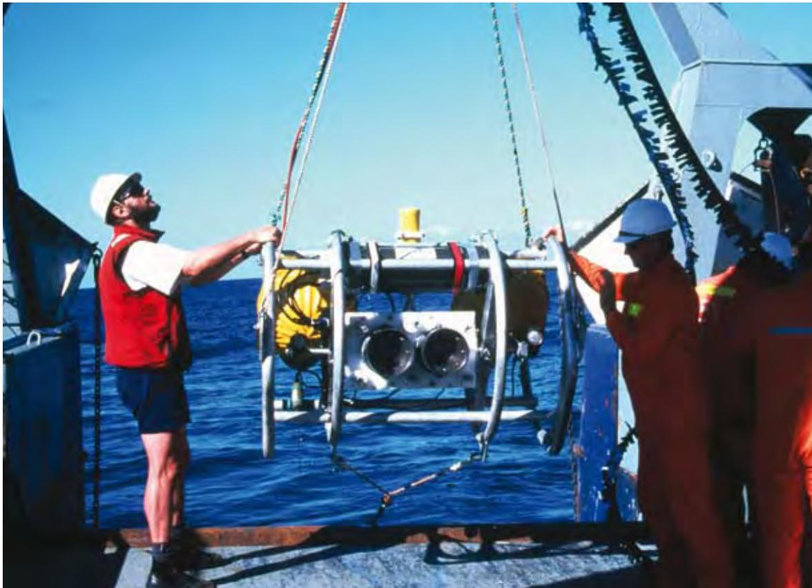
Scientists work on the deployment of the towed stereo video camera array, which is capable of working at depths of over 1500m, from the RV Southern Surveyor. Image courtesy of CSIRO.
