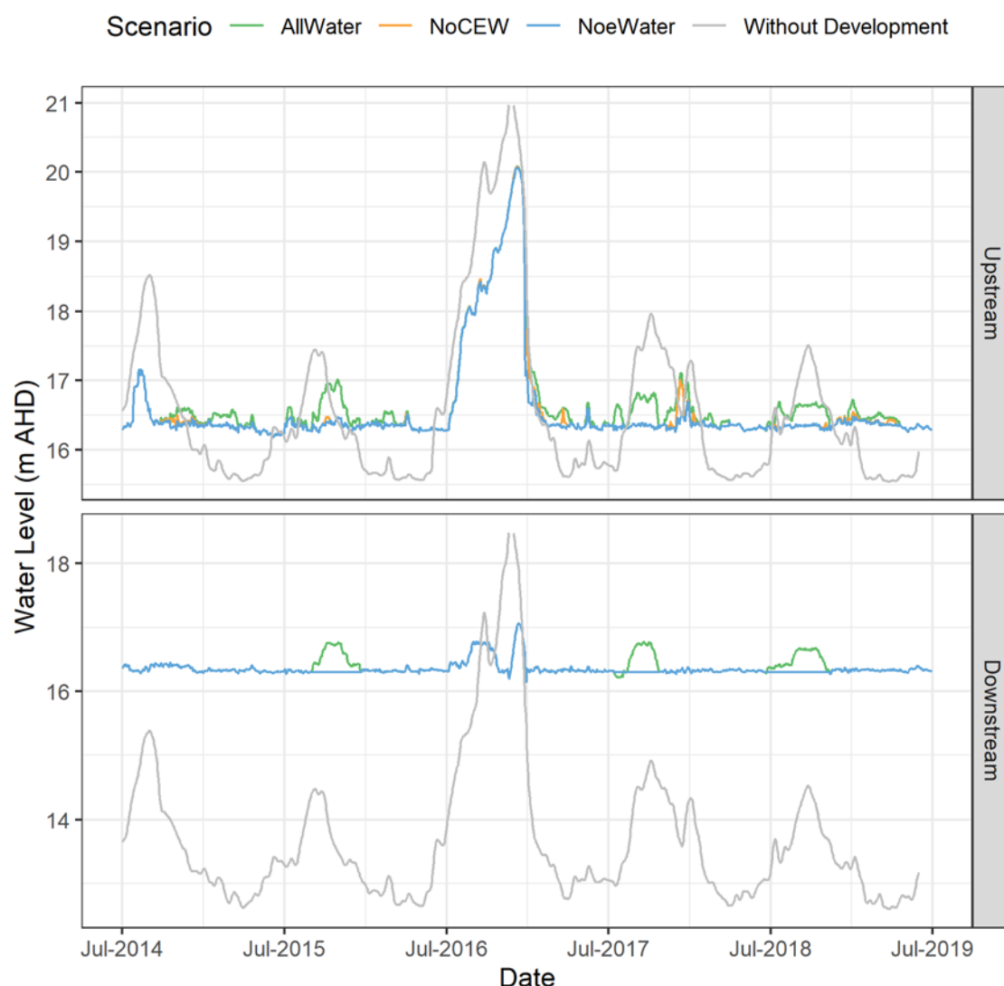
Figure 6. Modelled water level (metres relative to the Australian Height Datum) at the upstream and downstream end of the Lock 5 weir pool in the Lower Murray River. Coloured lines represent the modelled environmental water scenarios.
