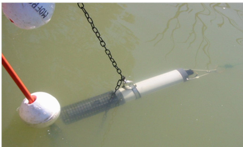
Figure 7. Loggers that are deployed in the Lower Murray River to measure dissolved oxygen concentrations (photo: University of Adelaide).
