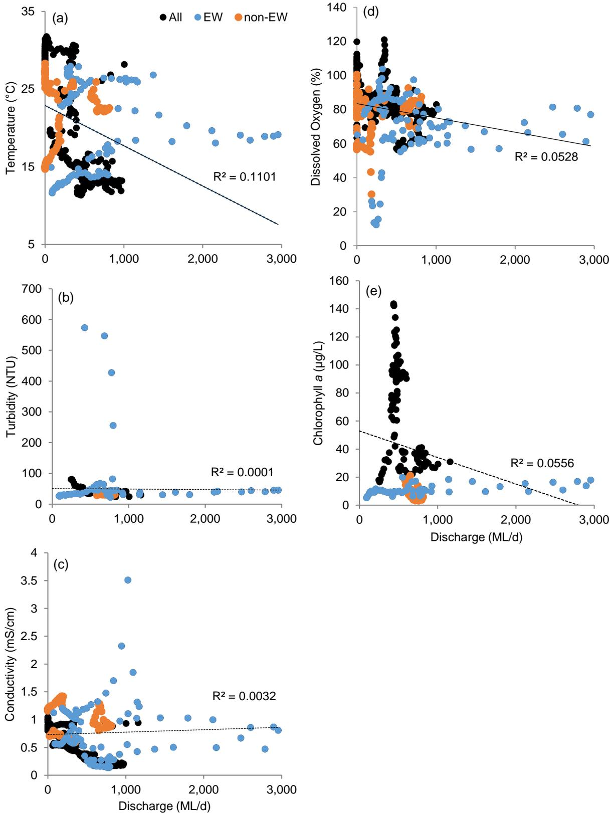
Figure E-7: Regressions between discharge at Darling @ Louth (NSW425004) on the Darling River system and mean daily (a) temperature, (b) turbidity, (c) conductivity, (d) dissolved oxygen concentrations and (e) chlorophyll a concentrations.
