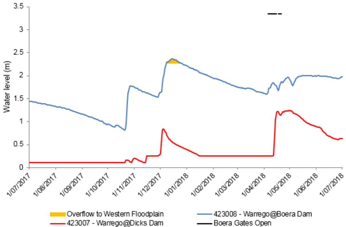
Figure A-1: Boera Dam levels during 2017-18 water year and flow to Western Floodplain and/or into lower Warrego channels (gates open).
