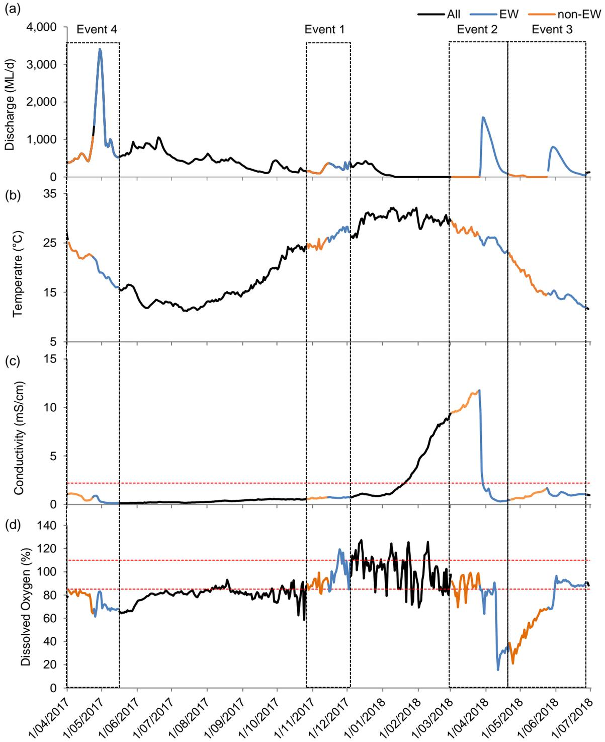
Figure E-4: Mean daily (a) discharge at Darling @ D/S Weir 19a (NSW425037) on the Darling River system, (b) temperature, (c) conductivity and (d) dissolved oxygen at Darling upstream water quality station. EW represents environmental water. Black line represents all available data from this watering year and red dotted line represents ANZECC guideline trigger value.
