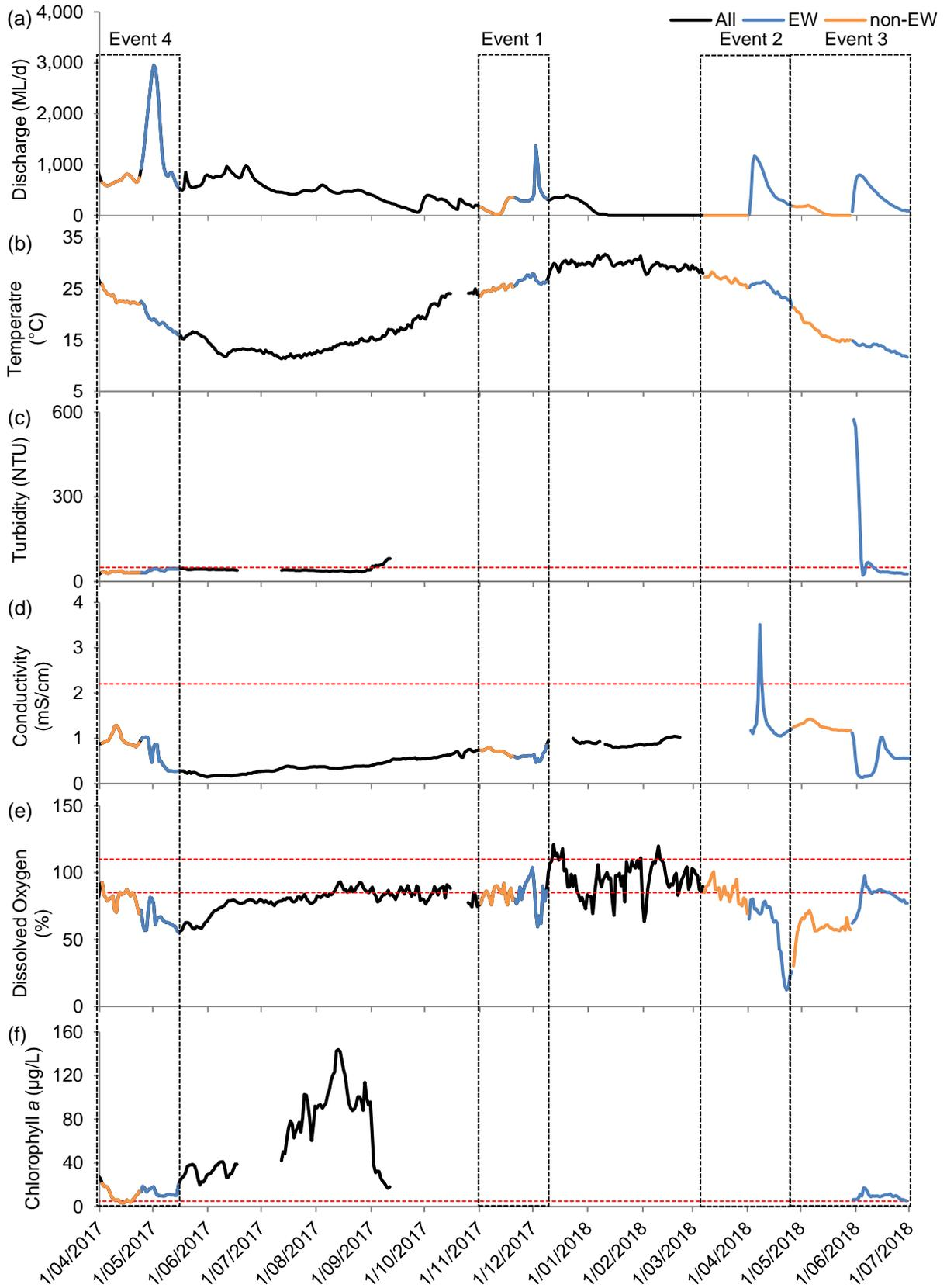
Figure E-5: Mean daily (a) discharge at Darling @ Louth (NSW425004) on the Darling River system, (b) temperature, (c) turbidity, (d) conductivity, (e) dissolved oxygen and (f) chlorophyll a at Darling downstream water quality station. EW represents environmental water. Black line represents all available data from this watering year and red dotted line represents ANZECC guideline trigger value.
