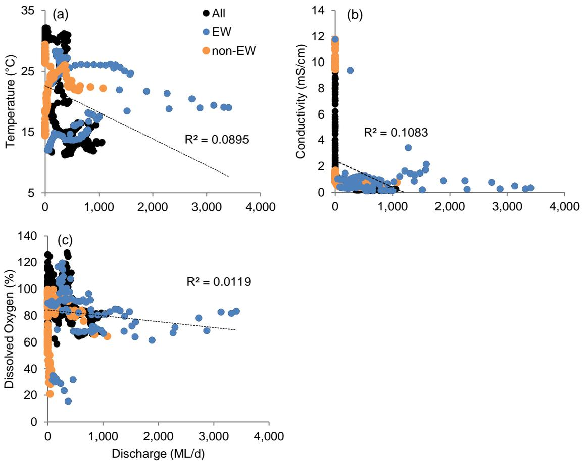
**Figure E-6: Regressions between discharge at Darling @ D/S Weir 19a (NSW425037) on the Darling River system and mean daily (a) temperature, (b) conductivity and (c) dissolved oxygen concentrations.**
