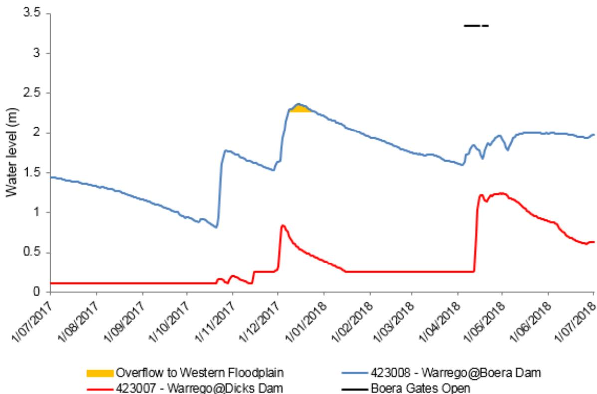
Figure G-1: Boera Dam levels during 2017-18 water year and flow to Western Floodplain and/or into lower Warrego channels (gates open).
