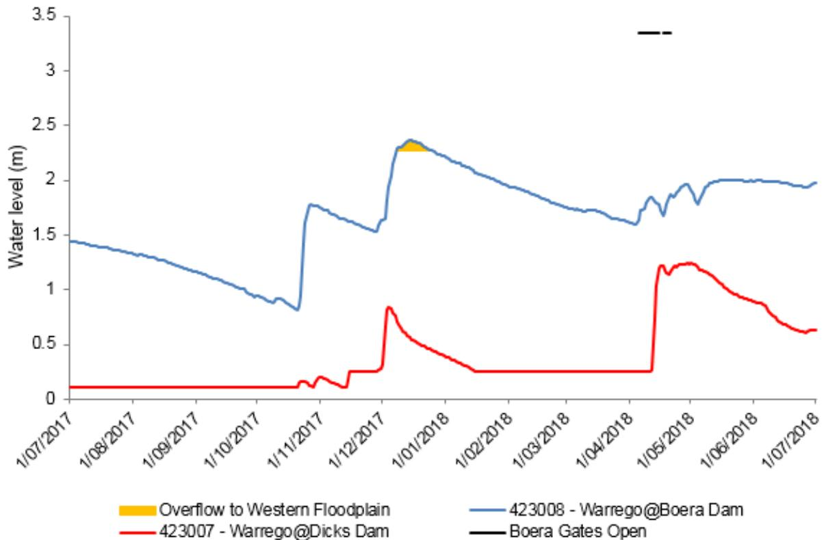
Figure H-1: Boera Dam levels during 2017-18 water year and flow to Western Floodplain and/or into lower Warrego channels (gates open).
