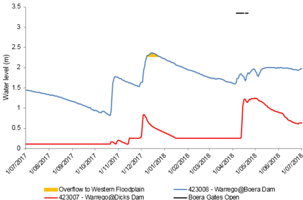
Figure F-1: Boera Dam levels during 2017-18 water year and flow to Western Floodplain and/or into lower Warrego channels (gates open).
