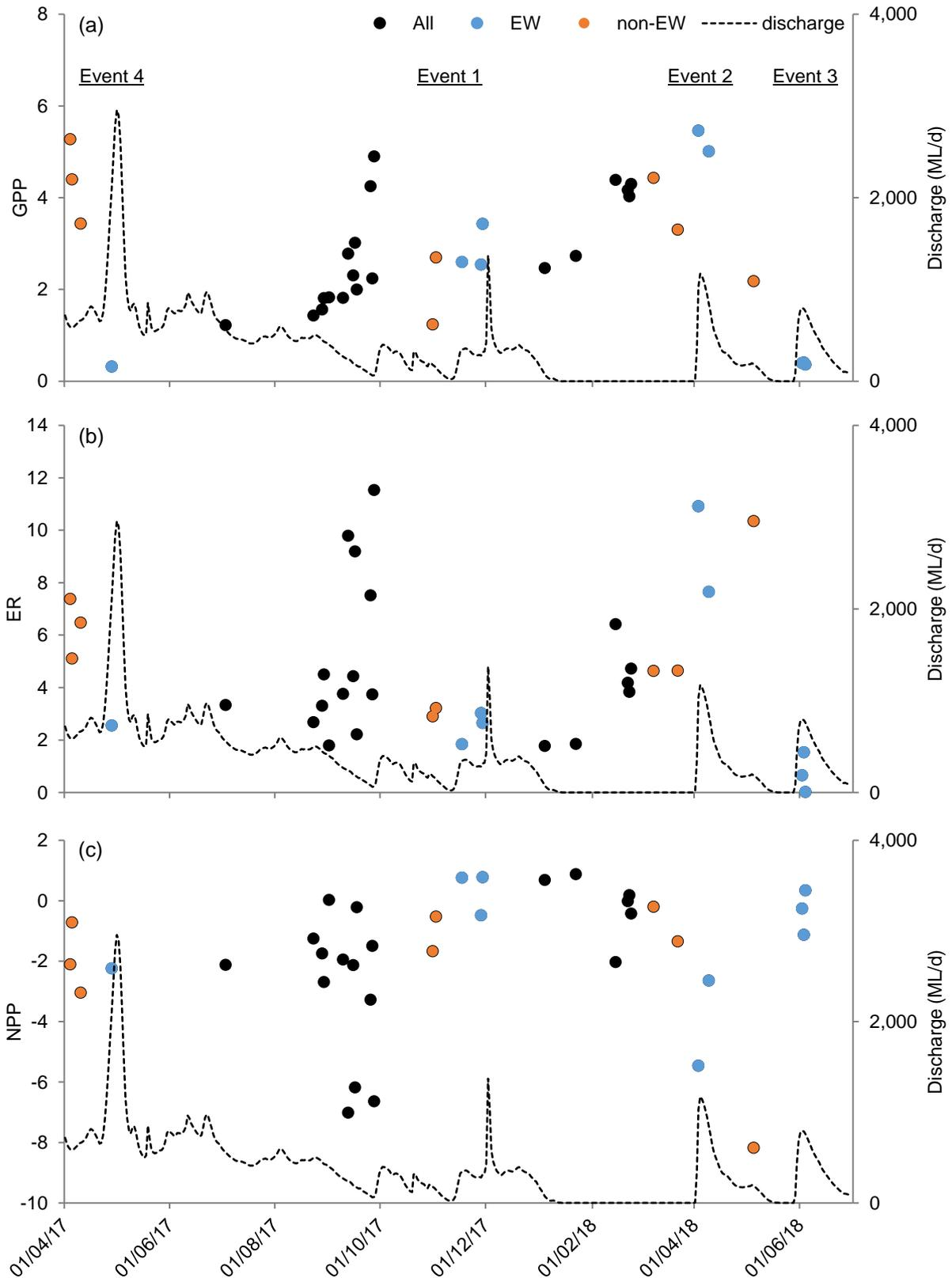
Figure F-5: Mean daily (a) gross primary production, (b) ecosystem respiration and (c) net primary production at Darling downstream stream metabolism station. EW represents environmental water. Black dotted line represents discharge (ML/d) data from the nearest gauge station Darling @ Louth (NSW425004).
