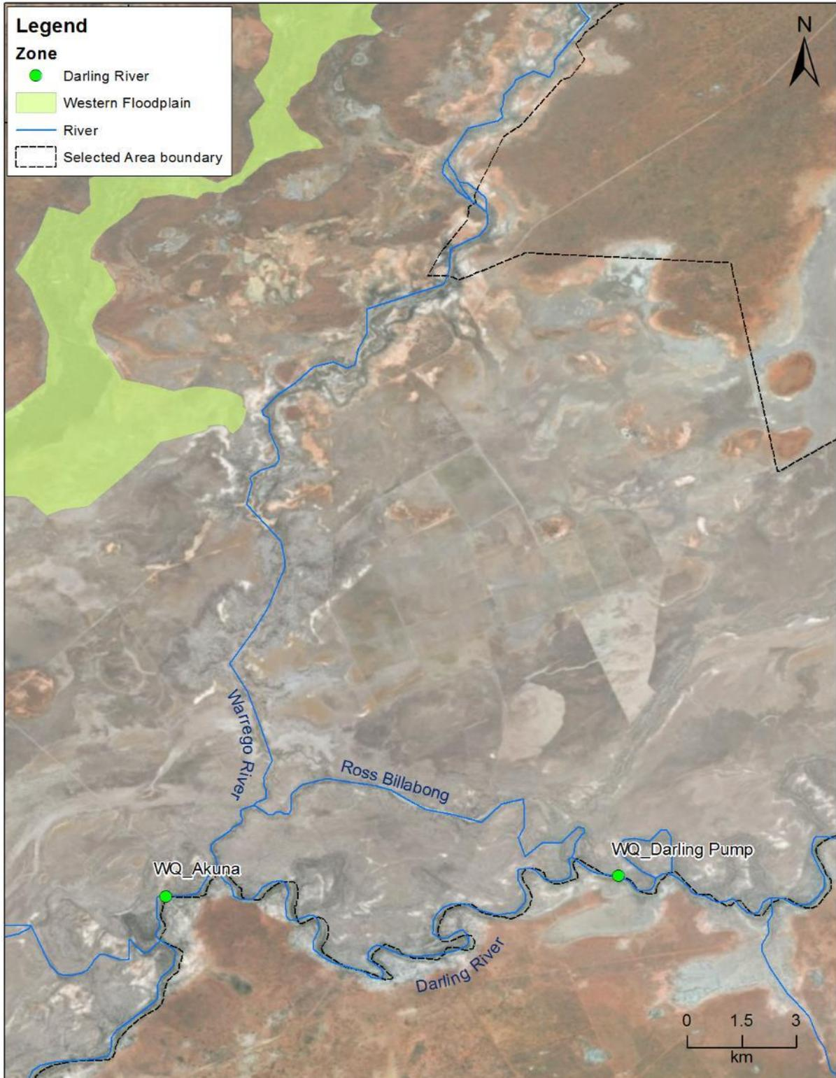
Figure F-2: Location of two long-term stream metabolism monitoring stations (Cat I) in the Darling River within the Selected Area. WD\_Darling Pump is the upstream station and WD\_Akuna is the downstream station.
