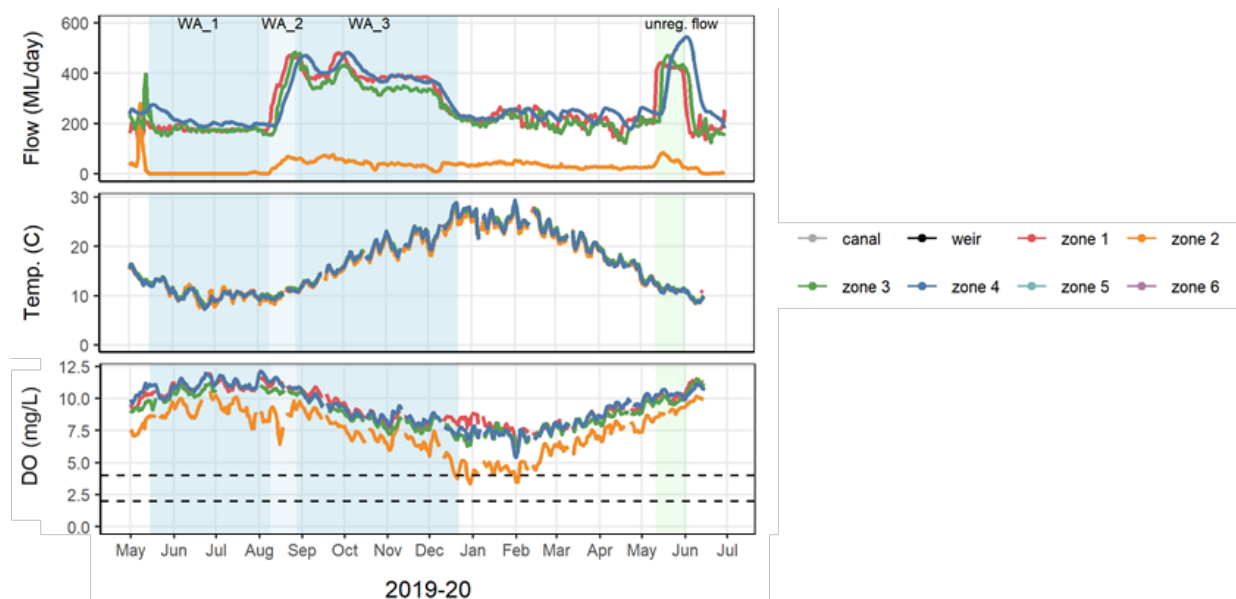
Figure 8. Daily discharge (ML/day), temperature (°C), and dissolved oxygen (DO) concentrations (mg/L) at sites in the Wakool-Yallakool system from May 2019 to June 2020. Dashed lines indicate DO range of concern for fish. Many fish species become stressed when DO is below 4 mg/L, and fish deaths can occur when DO is less than 2 mg/L.
