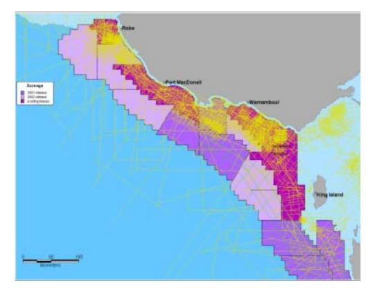
Fig. 18: Seismic surveys conducted in Otway Basin (yellow: 2D, green 3D), overlaying the acreage releases. Data supplied by GA
