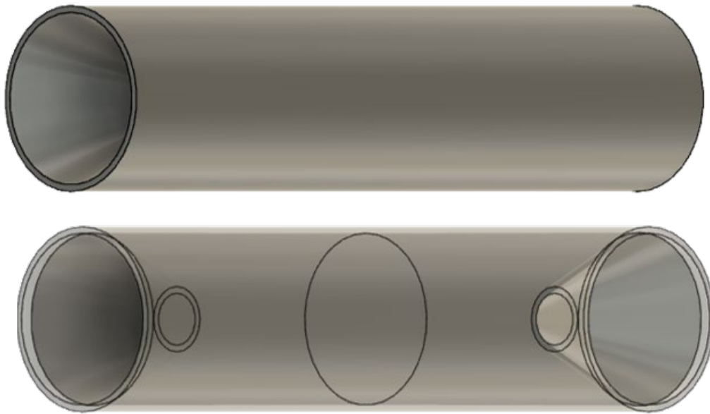
Figure 5: Model of cylindrical funnel trap used for amphipods. Bait is secured on the inside of the tube. Funnel opening is 10cm and internal end of funnel is 4 cm. NB: image is not to scale.
