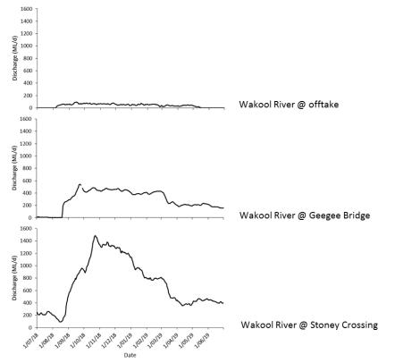
**Figure 4.4** Hydrographs for the Wakool River at offtake (gauge 409019), Gee Gee Bridge (gauge 409062), and at Stoney Crossing (gauge 409013) from 1 July 2018 to 30 June 2019.
