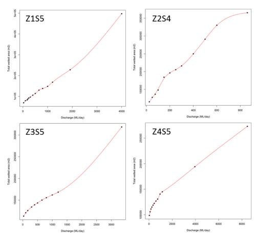
**Figure 4.1** Examples of relationship between discharge (ML/d) and total wetted benthic area (m<sup>2</sup>) for three of the nineteen 4 km reaches in the Yallakool-Wakool system. Estimates of wetted area were calculated from 2D hydraulic models. Curves were modelled using cubic smoothing spline regression approach, and were used to estimate the daily wetted area in each reach for each daily discharge during the flow trial.
