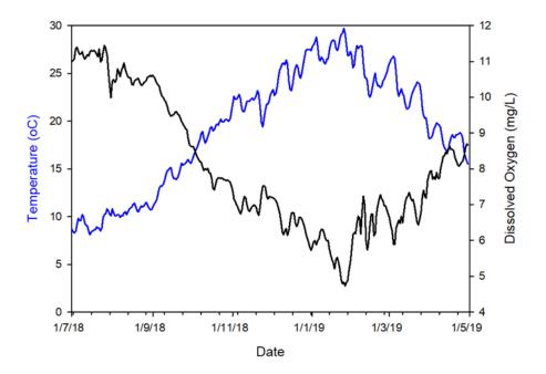
**Figure 5.11** Dissolved oxygen concentration (mg/L) and temperature (°C) in the Niemur River at the Barham Moulamein Rd (Data: Water NSW).
