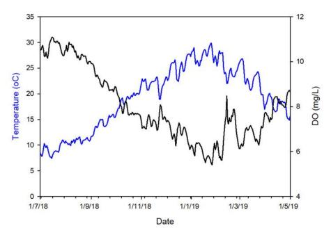
**Figure 5.12** Dissolved oxygen concentration (mg/L) and temperature (°C) in the Niemur River at Mallan School (data: Water NSW).
