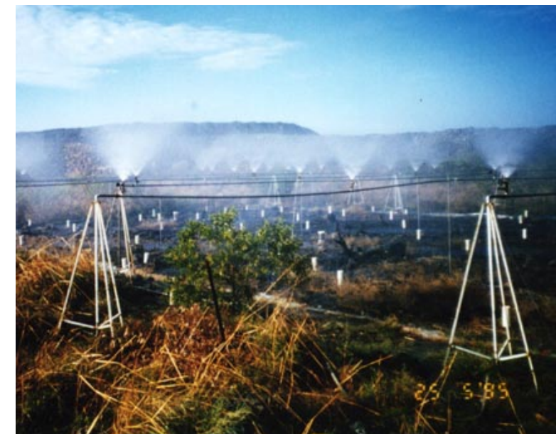
A large scale rainfall simulator being used at the Ranger mine by eriss researchers to collect sediment loss and runoff data for use in the SIBERIA model.
