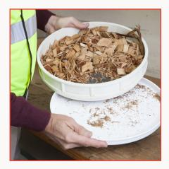
Examine the surface of the woodchips to identify any pests or contaminants that have not passed through the sieve.
