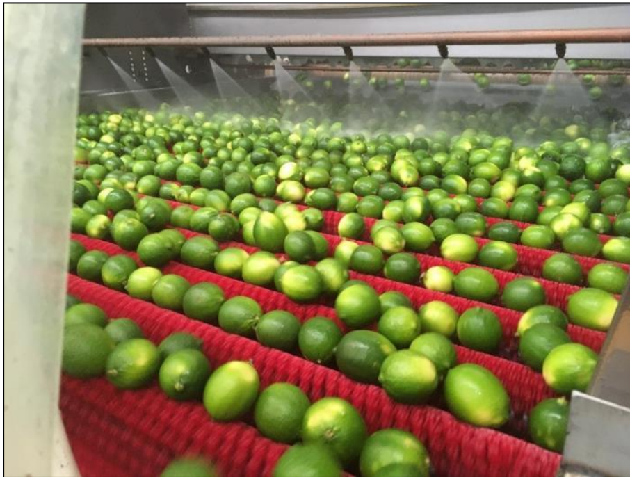
Figure 6 Soaping, washing and brushing stage
