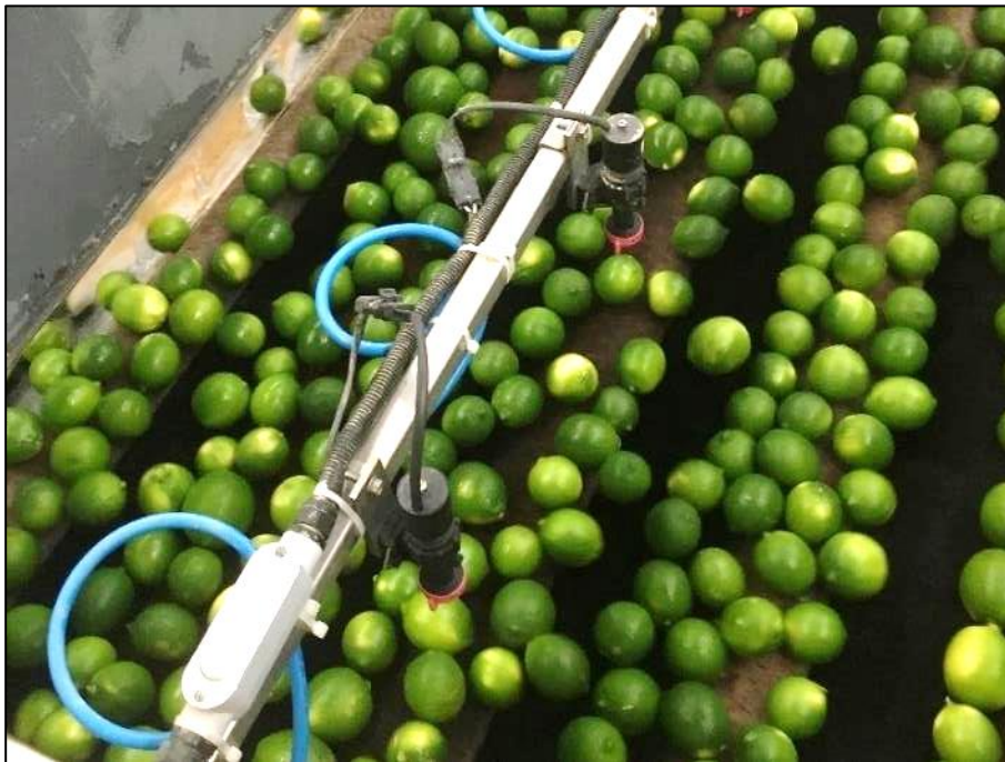
Figure 8 Application of wax in a fine mist via nozzles
