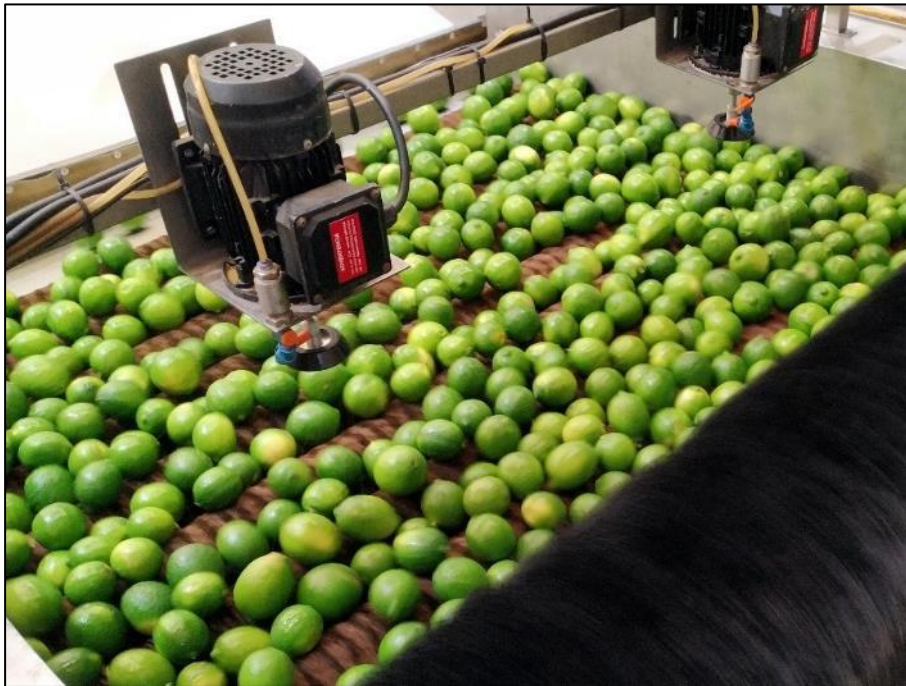
Figure 9 Application of wax on rotating disc
