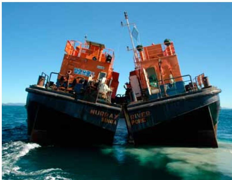
Split hull hopper dredge working on the Hay Point expansion project
