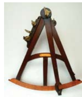
above: The Hadley octant, designed by John Hadley in 1731. This mahogany model was made by the famed London instrument maker, George Adams, in 1760.
