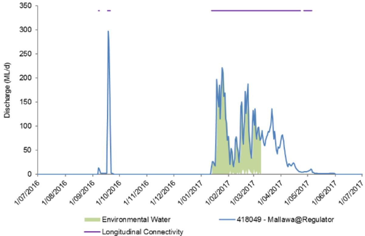
Figure A-7: River flows in Mallowa Creek and the timing of environmental water releases and 'wet' periods in this channel.
