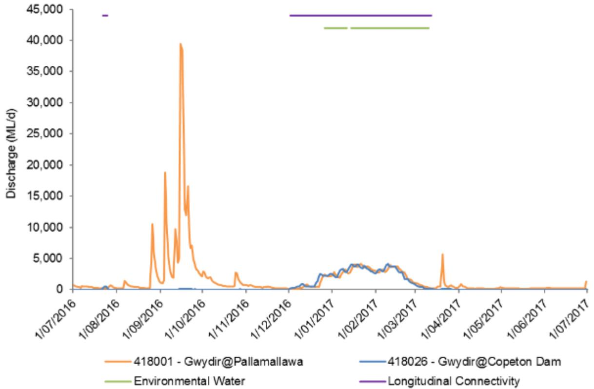
Figure A-2: River flows in the Gwydir River and the timing of environmental water releases and longitudinal connectivity down this channel.
