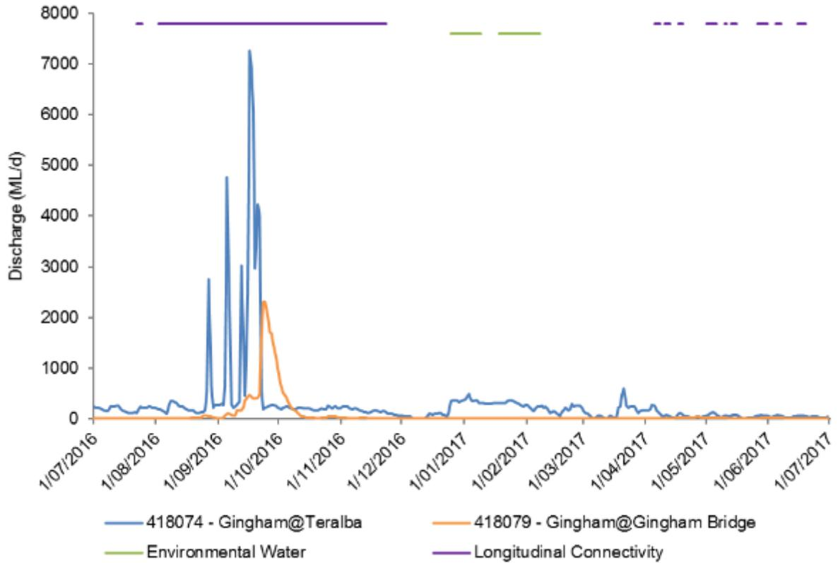
Figure A-4: River flows in the Gingham Watercourse and the timing of environmental water releases and longitudinal connectivity down this channel.
