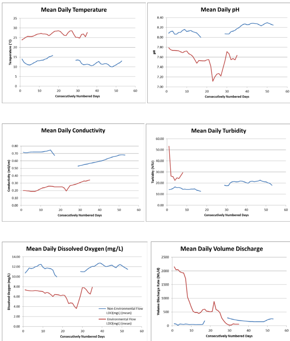
Figure F-1: Mean daily temperature (°C), pH, Turbidity (NTU), Salinity (mS/cm) and Dissolved oxygen (mg/L) at the Pallamallawa gauge (NSW418001) in the Gwydir River. Blue indicates Non-environmental water delivery and red indicates environmental water delivery.
