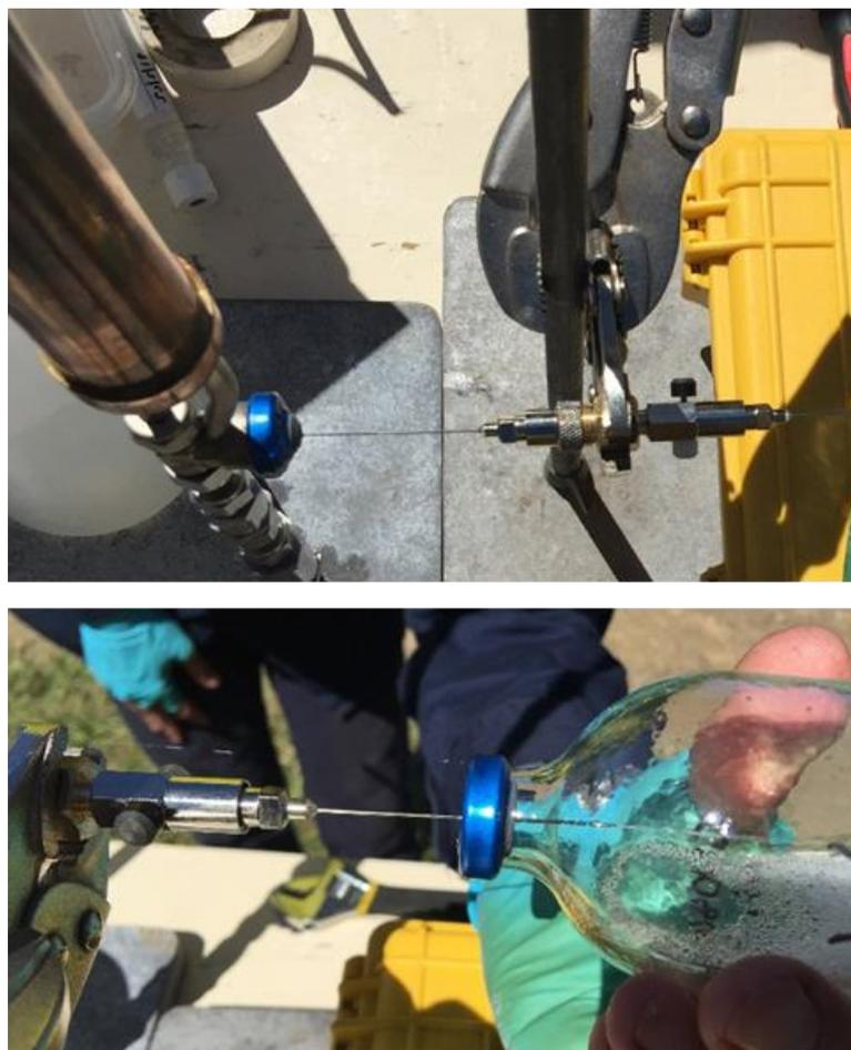
**Figure A-3 Sample collection in the field using a double ended syringe from the butyl-rubber septa sample port of the downhole sampler.**
