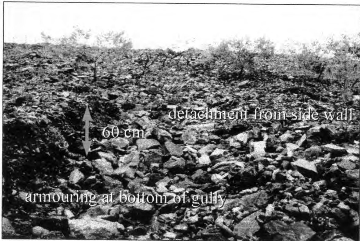
Figure 3.2.18: The excavation of material from Row H to Row I, reaches a depth of 60cm with large rock fragments armouring further incised.
