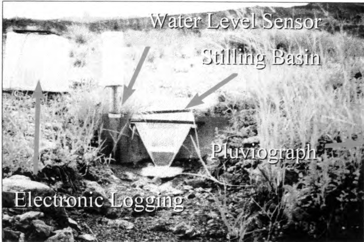
Figure 2.1: A standard 150mm flume was re-commissioned and used for monitoring hydrological data for the study site. Discharge recorded from the cap site area 591\text{m}^2 , together with cumulative rainfall was used to calibrate the hydrology model DIST-FW, and hence characterise each of the storm events.
