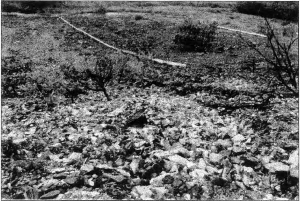
Figure 3.2.11: The removal of fine material was more widespread below Row D, as seen by the painted fluorescent lines across the slope. Both channels combined, and the gully pathway was not easily discernible.
