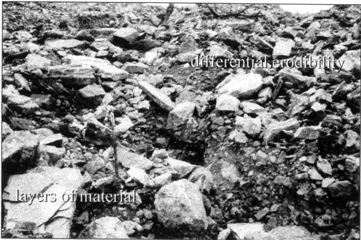
Figure 3.2.17: The depth of erosion reached 60cm in some places, revealing the heavily armoured rock fragment layer. The differential erodibility of these surfaces is considered with the soft earthen material extracted from above the mined ore seen as brown colour. Depth-erodibility relationships for this slope would therefore be complex, once the protective layer is breached.
