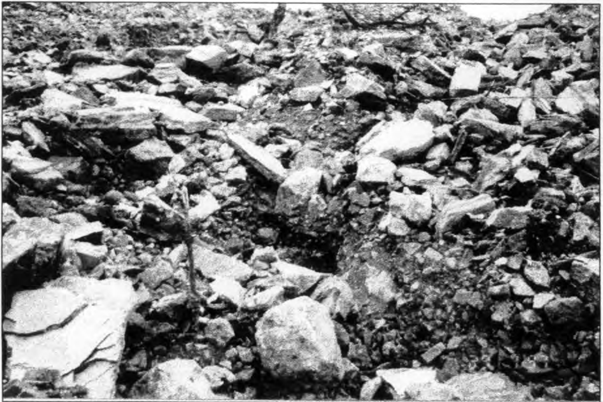
Figure 2.7: The erodibility of the waste rock material was dependent on the mean grain size, relative weathering and overall rock consistency. Erosion pins used, were considered ineffective, with excavation of gully reaching 50 to 60cm in places removing these devices.
