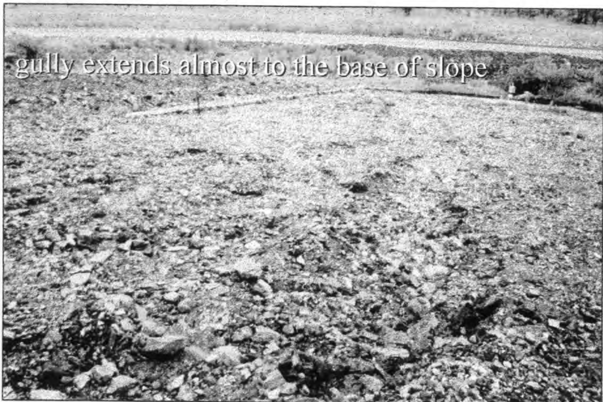
Figure 3.2.19: The gully extends to Row I with depth of 20cm to 30cm, whilst almost reaching the concrete apron of the flume pictured in background.
