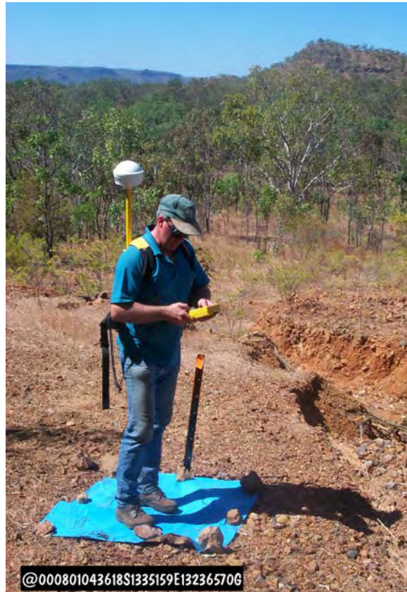
Plate 1. Images were registered to Ground Control Points using a Trimble™ dGPS. GCPs were distributed regularly throughout sites and were also placed at each end of permanent transect lines (Guratba site, lower slopes).
