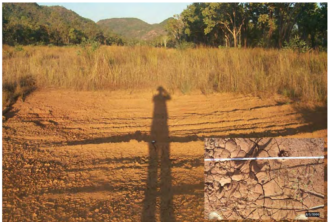
Plate 7. Lateritic clay/silt was typically deposited in poorly drained depressions at airstrip. These areas were used as training sites from which the 'clay/silt' class were formed in the supervised classification procedure.
