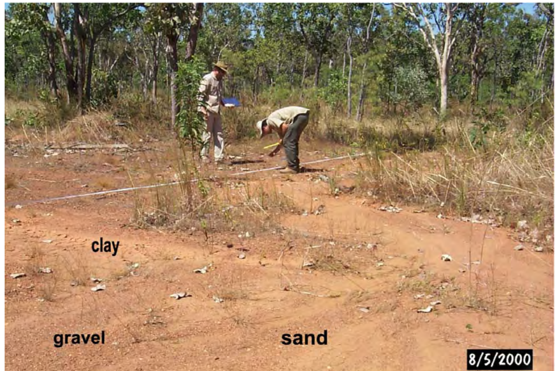
Plate 6. Gravel, sand and clay were deposited in different regions, disproportionately, relative to runoff/erosive characteristics created by micro-topographical features along the gentle slope of the airstrip. Sandy areas formed a characteristic zone representing erosion deposits transitional between lag gravel on steeper runoff areas and clay in poorly drained, seasonally waterlogged areas.
