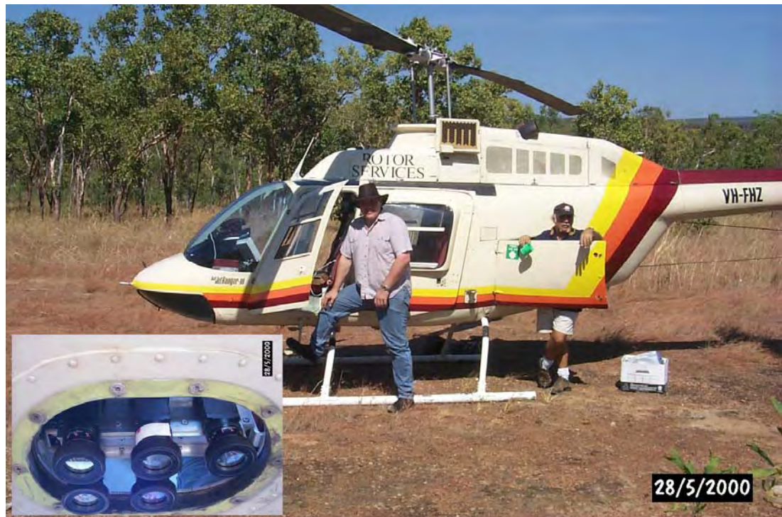
Plate 3. The 5-camera ICU array was fitted to the undercarriage of a Bell Jet-ranger helicopter.
