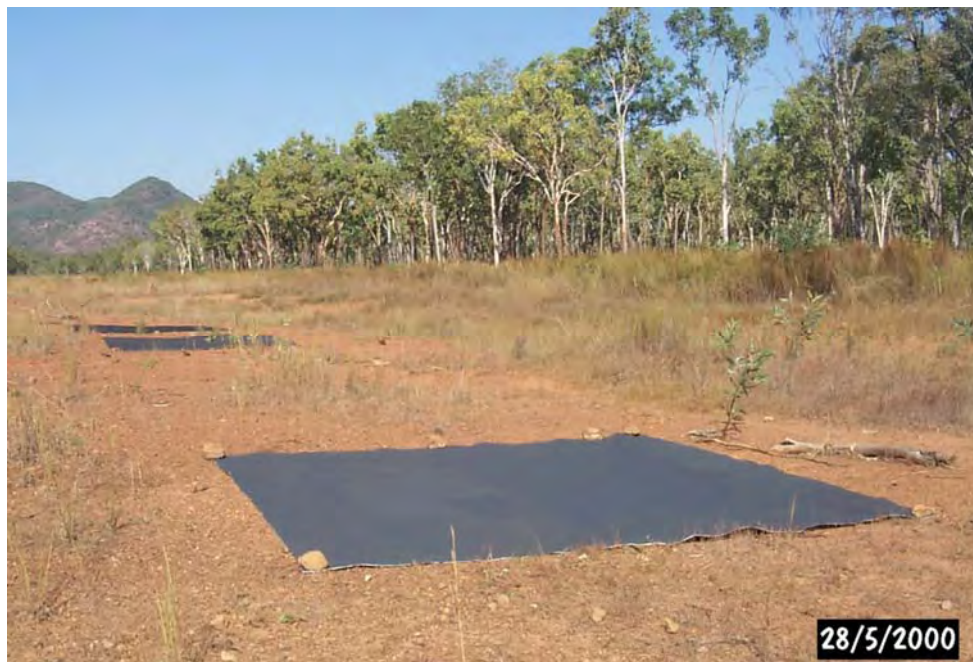
Plate 2. Canvas 3x3 m spectral calibration targets were deployed at the airstrip site to allow imagery to be standardised to ground reflectance measurements.
