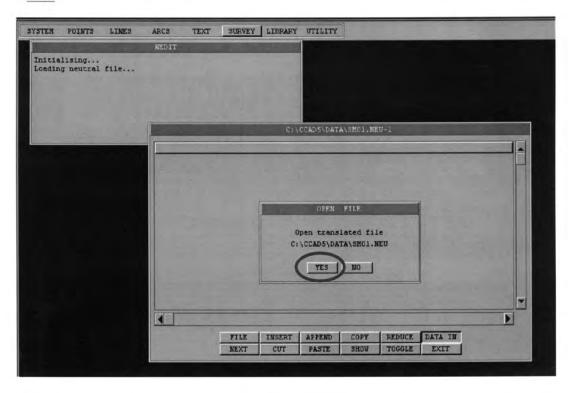
(p) Data will now be loaded into the neutral editor. To ensure data is in correct format to import into Excel it must be saved again and the .neu file is overwritten.
