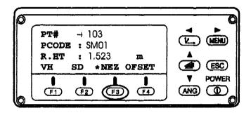
(f) Repeat steps (d) and (e) until survey has been completed then <u>ESC</u> This will signal to the machine that the survey of the job has been completed. The machine can now be turned off or a new job can be entered.
