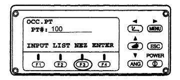
(d) <u>F1 INPUT</u> Input N (northing), E (easting) and Z (elevation) values for the set up point and press <u>F4 ENTER</u> after each entry.
