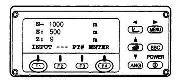
(e) After inputting the z value and hitting the enter key the screen will revert back to previous screen shown below. Occupied station details have now been completed. Hit <u>ESC</u> to get to the next screen.
