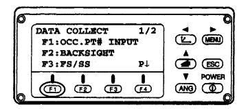
(b) F1 Input point number for occupied point.(set up point) Use 100 for all occupied point numbers.
