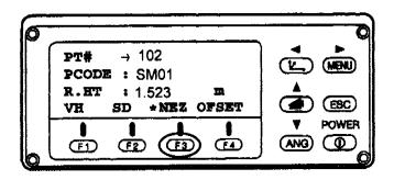
(d) A series of beeps means the point has been taken. The staff can now be moved to the next point. The screen will be the same as below. Note that the point number has increased by one - the total station will do this automatically for each survey point until the pickup has been completed. To continue the survey F3 MEAS If you need to change the point code or prism height for a particular survey point this can be done by using the F1 INPUT key and F4 ENTER keys. Then F3 MEAS
