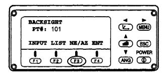
(d) For surveying cross-sections a backsight bearing is generally used. Press <u>F3 AZ</u> and go to step (e).
