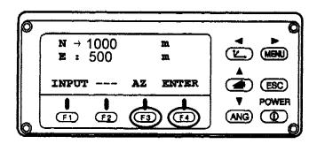
(e) <u>F1 INPUT</u> Input the backsight bearing for the section.
