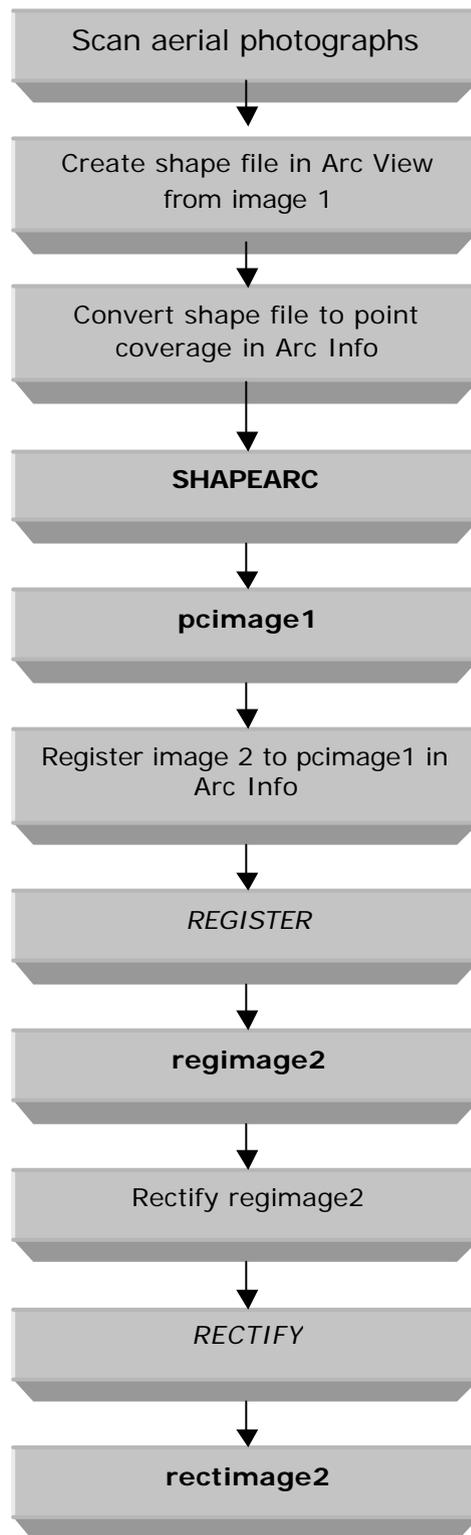
**Figure App-1 Example of Image-to-Image Registration and Rectification**
