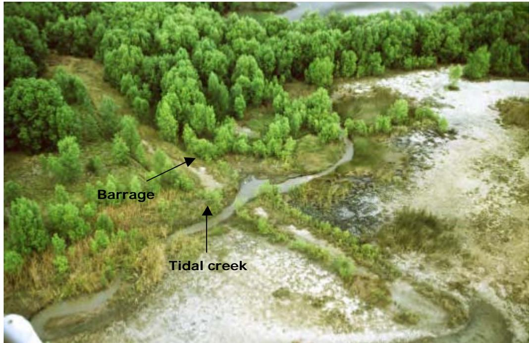
**Plate 2.1 Tidal Creek Outflanking Barrage**
