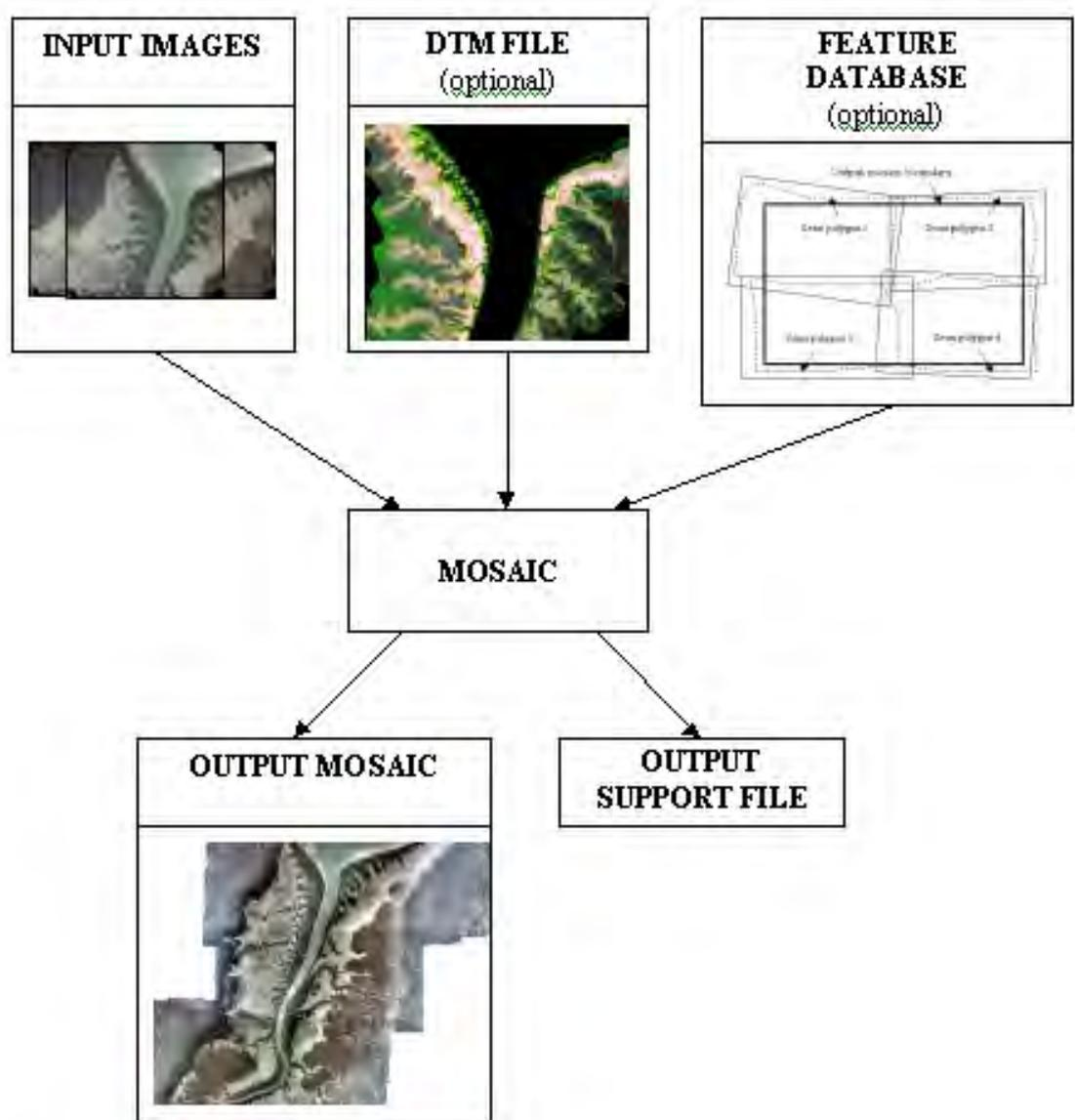
Figure 6. Flow chart outlining the generation of an orthomosaic. Typical inputs include one or more triangulated images, a DEM, a feature database of seam polygons (that define each image space), and an output boundary.
