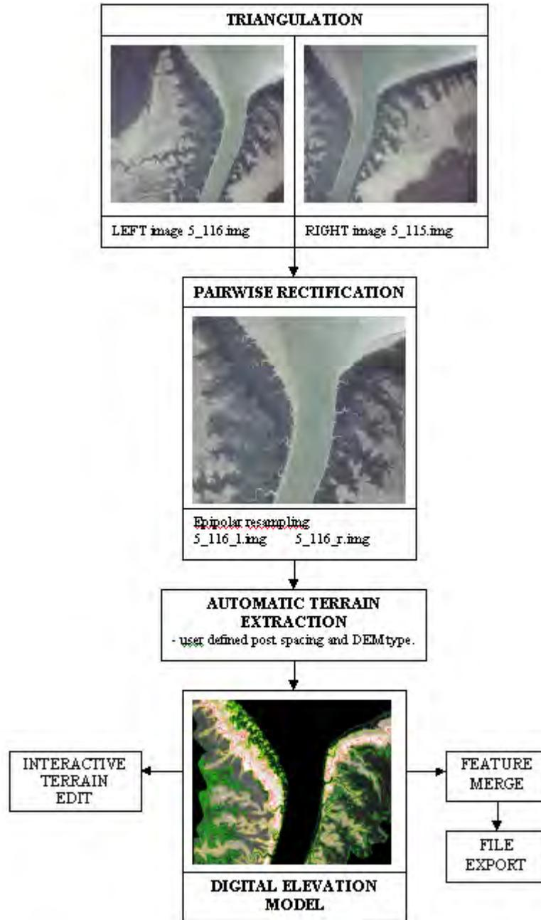
Figure 5. Flow chart outlining the DEM generation process whereby ATE is performed in the area of overlap of a stereo pair. User-defined options include the density of elevation points to be collected and the format of the data (grid, TIN triangles). The resulting DEM can be overlain on the stereo pair as continuous contours for editing as required.
