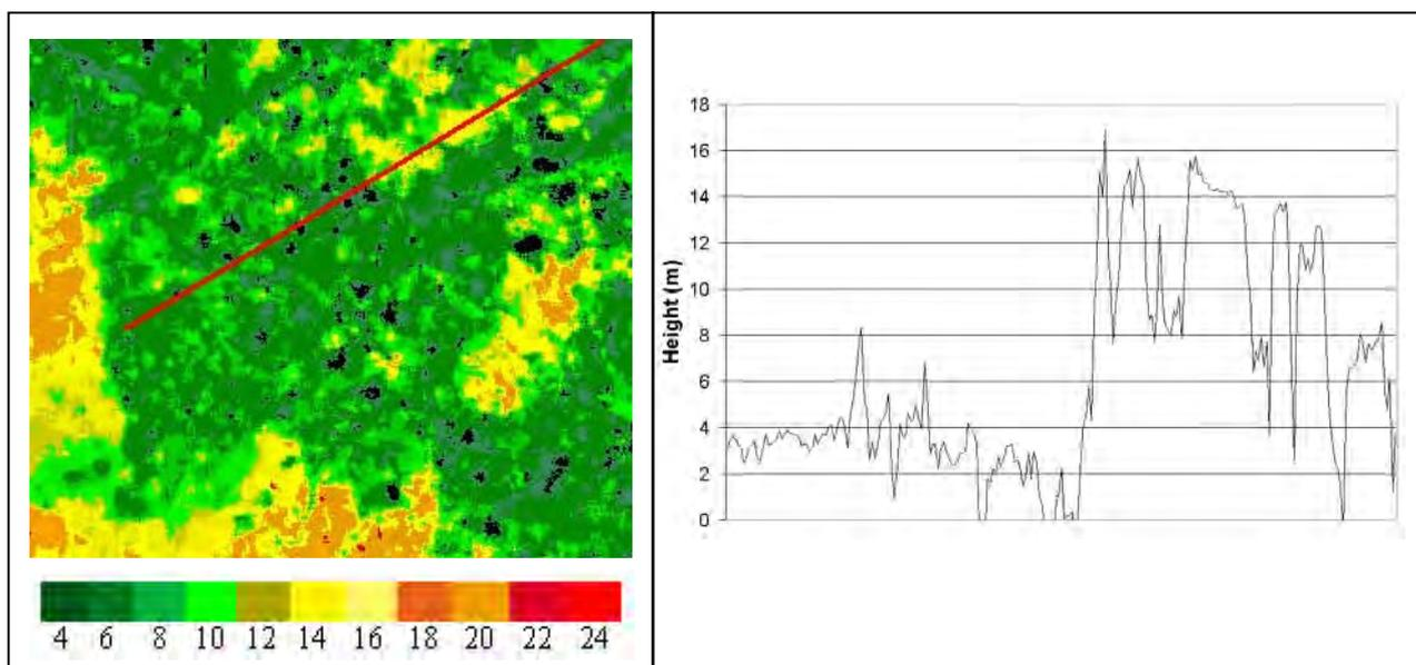
Figure 13. Inconsistencies in height estimation associated with DEM generation for open forest: a) 5 m DEM; and b) Profile extracted through mangroves.
