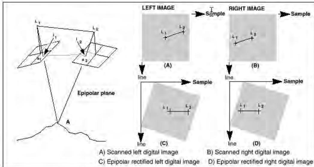
Figure 4. The image rectification process involving rotation along the epipolar plane and resampling of stereo pairs.
