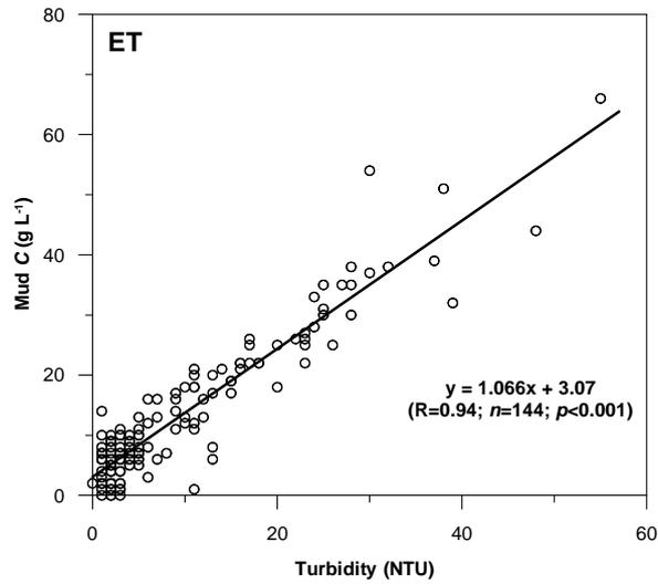
**Figure 3.2** Revised calibrated turbidity-mud C relationship for ET with outlier removed
