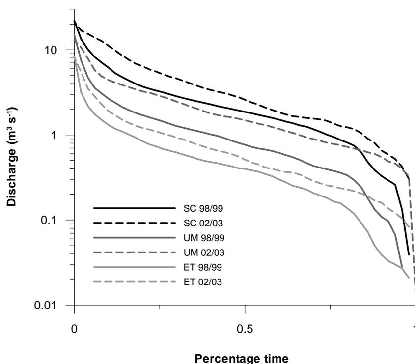
Figure 2.3 Standard flow duration curves for the Ngarradj catchment – 1998/99 and 2002/03
