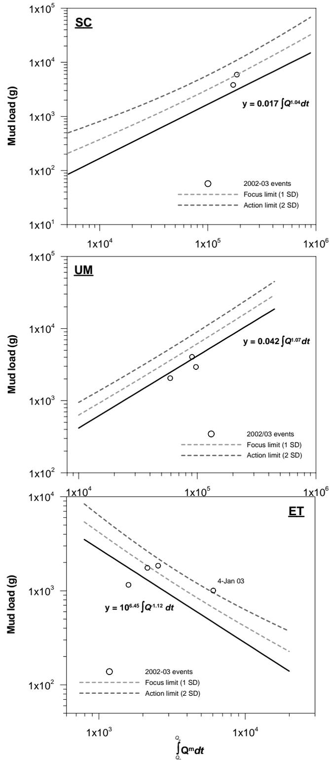
**Figure 3.6** Event-based mud load models for each gauging station. Observed event mud loads for 2002/03 are also shown.
