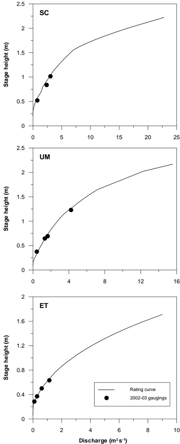
**Figure 2.2** Rating curves for SC, UM and ET with the gauging points take during 2002/03 shown
