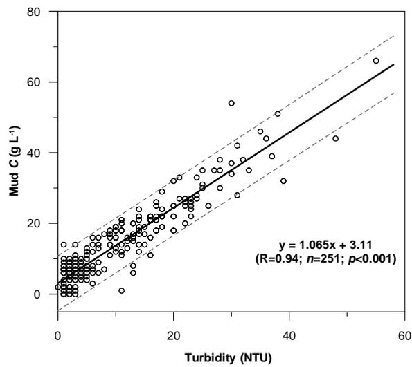
**Figure 3.3** Calibrated turbidity-mud C relationship for the combined data collected at UM and ET. 95% prediction limits for the regression equation are shown as dashed lines.
