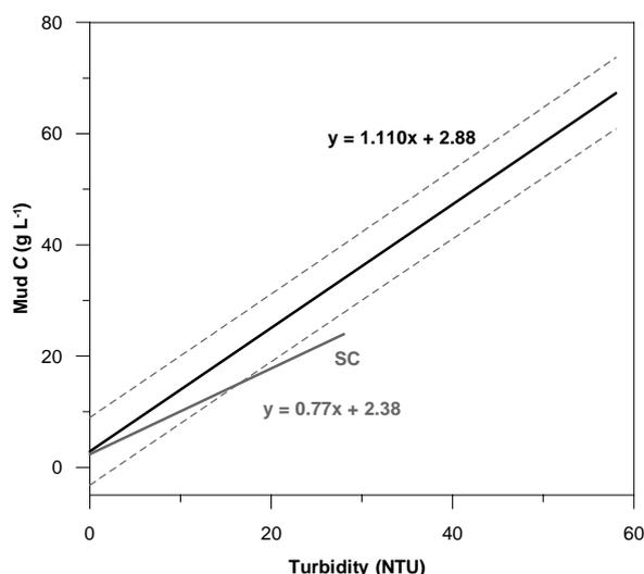
**Figure 3.5** Turbidity-mud *C* relationships fitted for data collected at SC and the combined data collected at UM and ET
