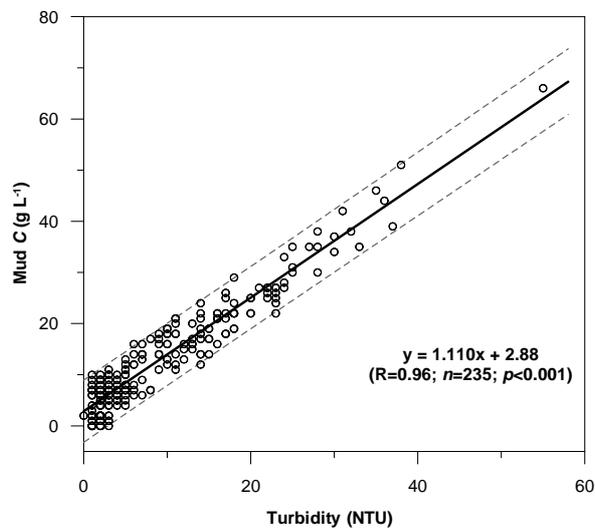
**Figure 3.4** Revised calibrated turbidity-mud C relationship for the combined data collected at UM and ET (outliers removed). 95% prediction limits for the regression equation are shown as dashed lines.
