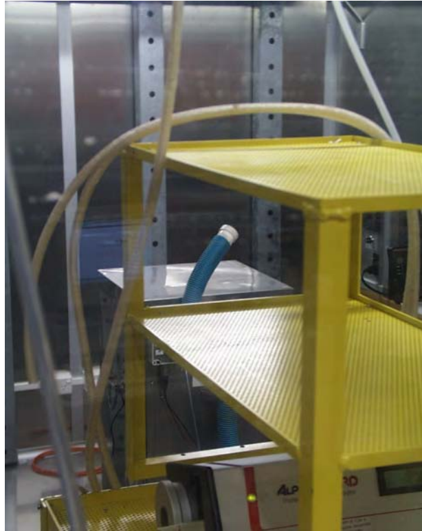
Figure 5 eriss 's radon monitor 1 in ARPANSA's radon chamber
