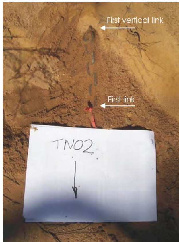
Figure 2 Scour chain at TN02 on 24 October 2000 orientated downstream. Arrow on paper shows flow direction.
