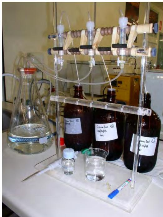
**Figure 7** Vacuum manifold apparatus used to pass plunge pool water samples through solid phase extraction columns
