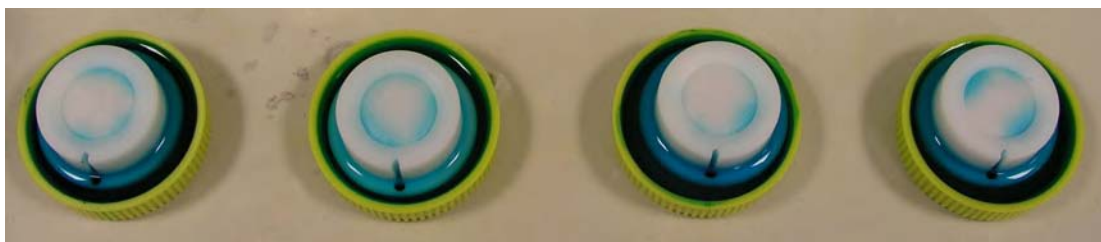
Figure 3.5 DGT casing loaded with tissue paper in place of the gel assembly at time = 8 hours.
