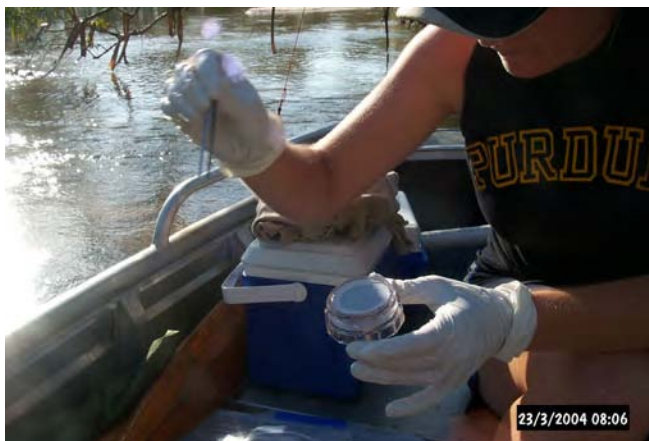
Figure 2.5 a) Filter apparatus preparation. b) Syringe filtration into 60 mL sampling bottle.
