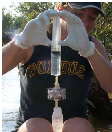
Figure 2.5 a) Filter apparatus preparation. b) Syringe filtration into 60 mL sampling bottle.
