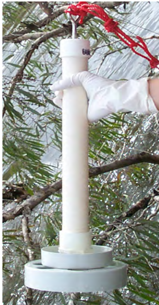
Figure 2.2 PVC DGT holder used for field deployment of DGT devices.
