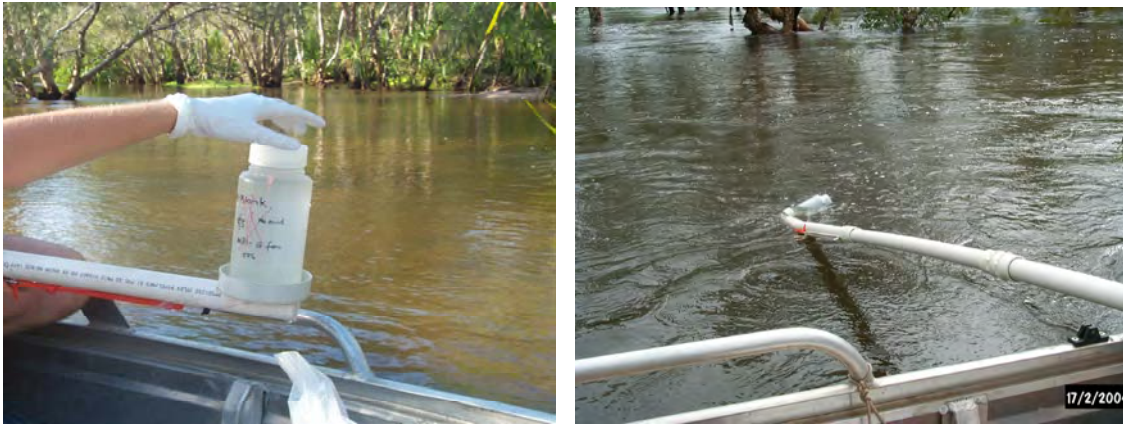
Figure 2.4 Collection of 1 L sample using sampling pole.
