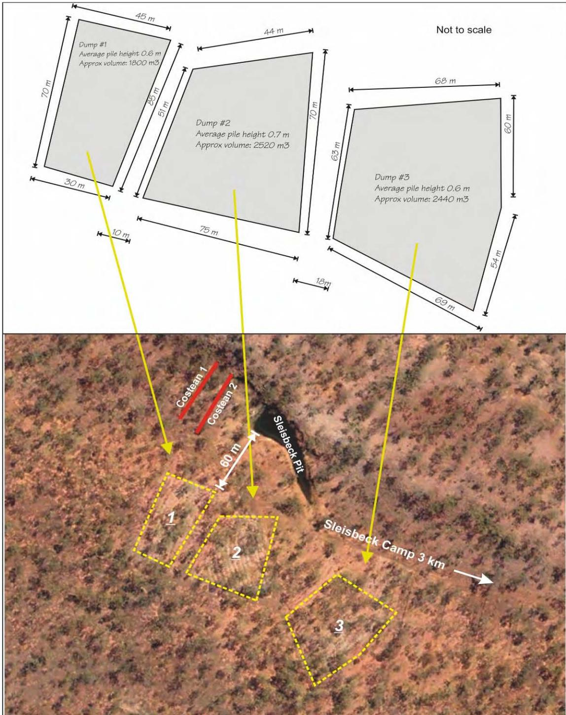
**Figure 7** Approximate location and extent of truck dumps 1, 2, and 3, respectively. Satellite data from Google Earth 2005.
