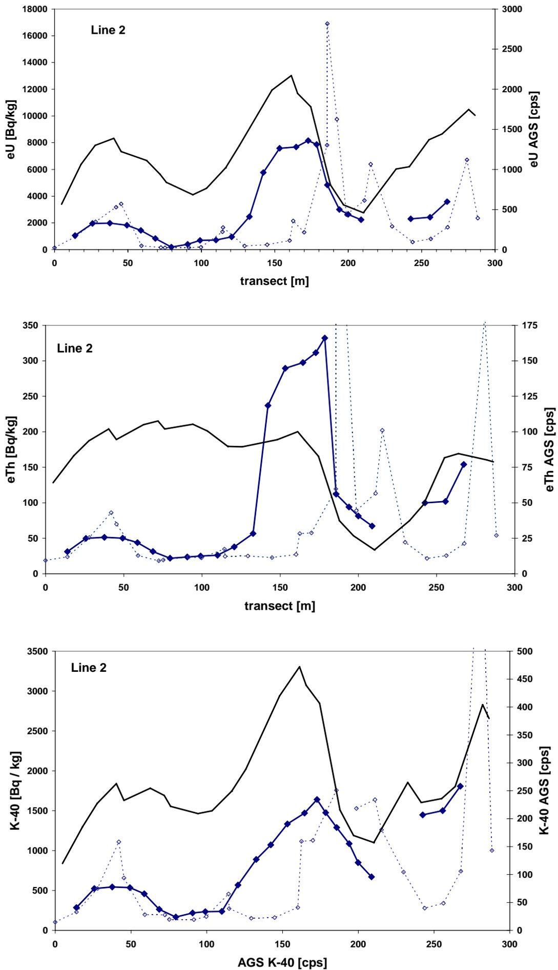
**Figure 15** eU, eTh and K-40 for Line 2 (dashed), smoothed and shifted data (solid), and associated AGS data (thick line)
