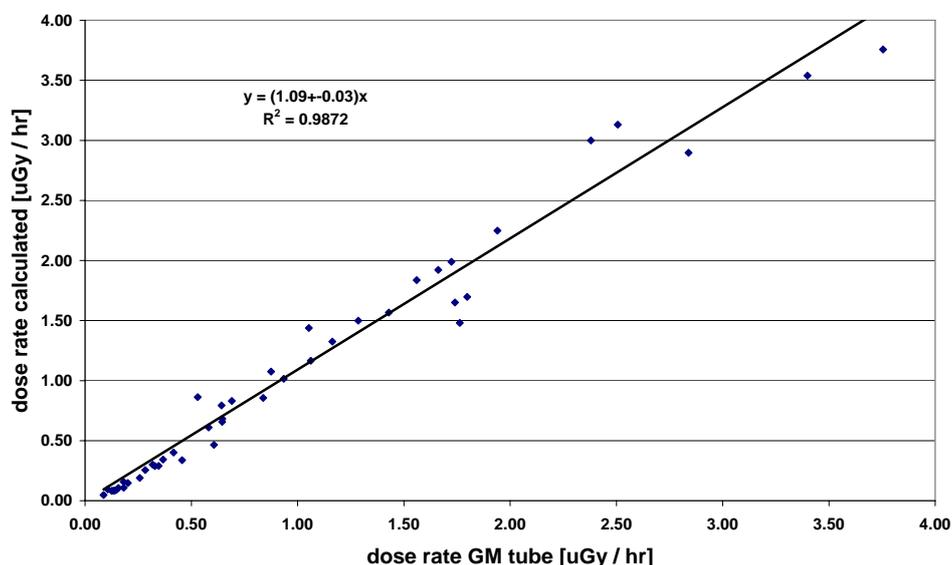
**Figure 17** Comparison of calculated (using equation 1) ground based and measured (using Mini Instruments, 6-80/MC-71 Environmental Radiation Meter) gamma dose rates
