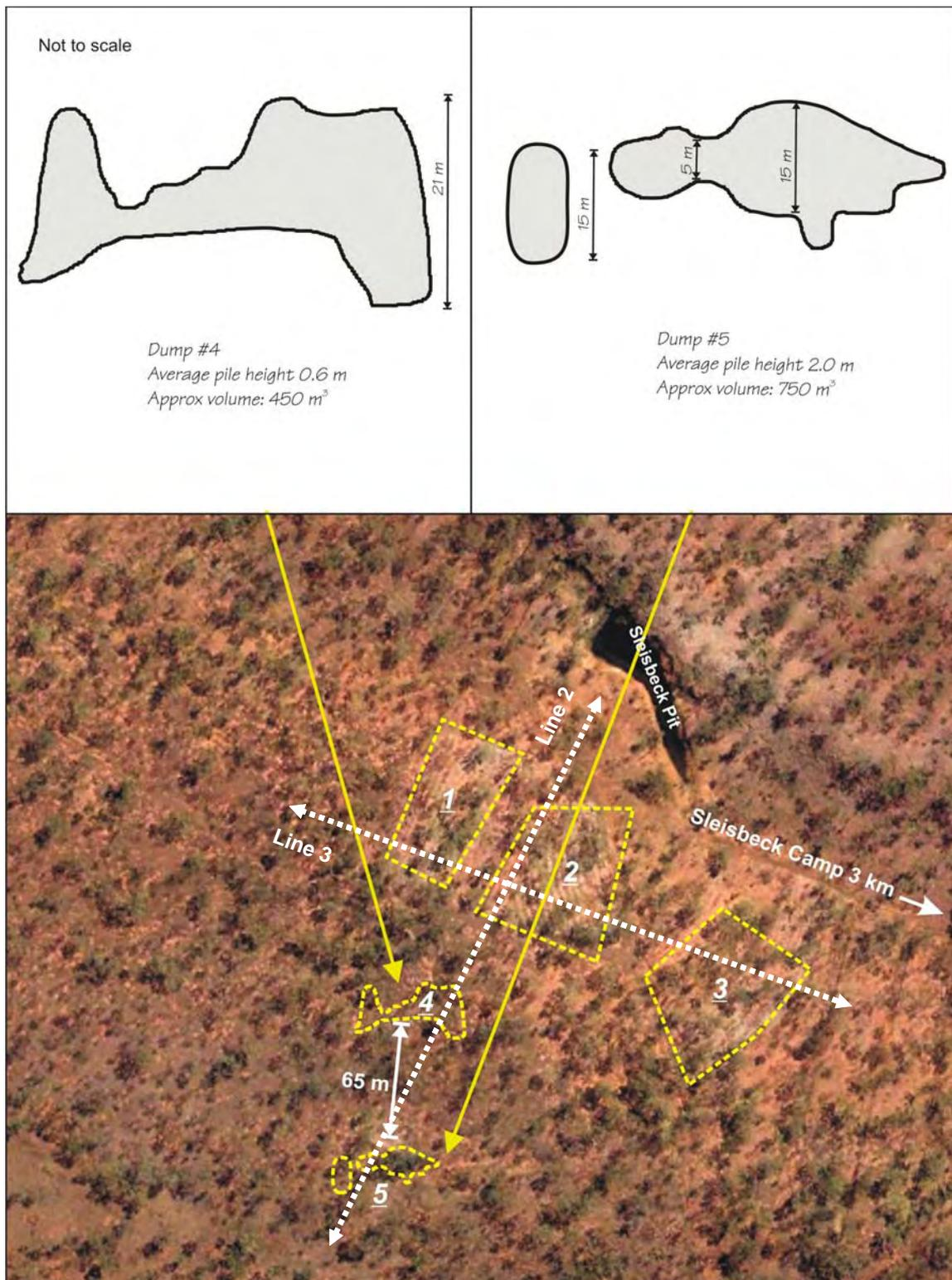
**Figure 8** Location and extent of truck dumps 4 and 5, and transect lines 2 and 3, respectively. Satellite data from Google Earth 2005.
