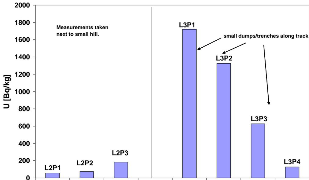
Figure 14 Equivalent uranium activity concentrations measured in 2003 at sites L2P1-L3P4
