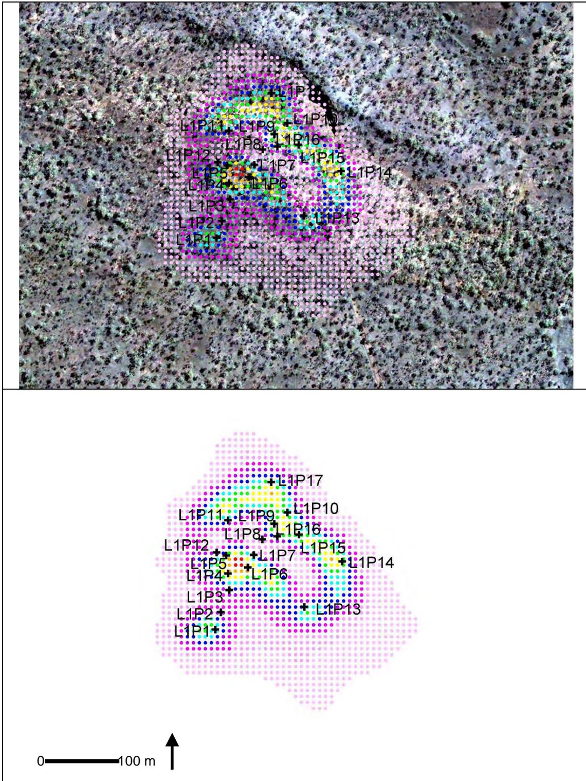
**Figure 11** Subset of Figure 4, highlighting the pit and low level dump areas, with airborne gamma > 200 counts per second overlaid, and the location of the 2003 groundbased measurements
