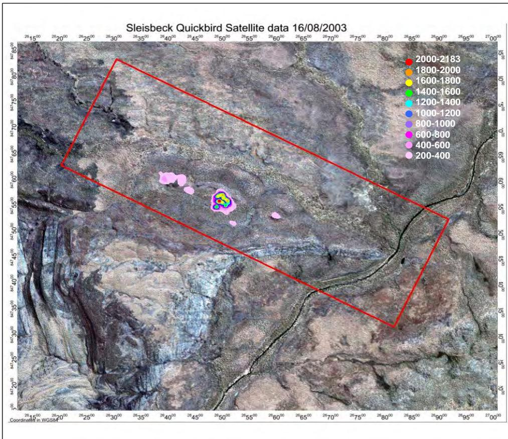
**Figure 5** Quickbird satellite data coverage with airborne gamma > 200 counts per second overlaid
