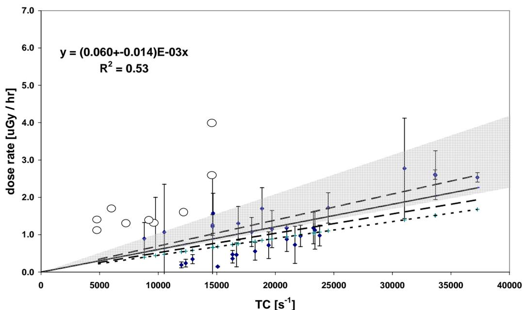
**Figure 18** Airborne total gamma counts versus measured gamma dose rates on ground. Positive outliers (open circles, 3-sigma indicated by the shaded area) from the ground survey have been removed and the remaining data points used to derive the slope (solid) and 95% confidence interval (dashed). Error bars show one standard error of the mean of the groundbased measurements.
