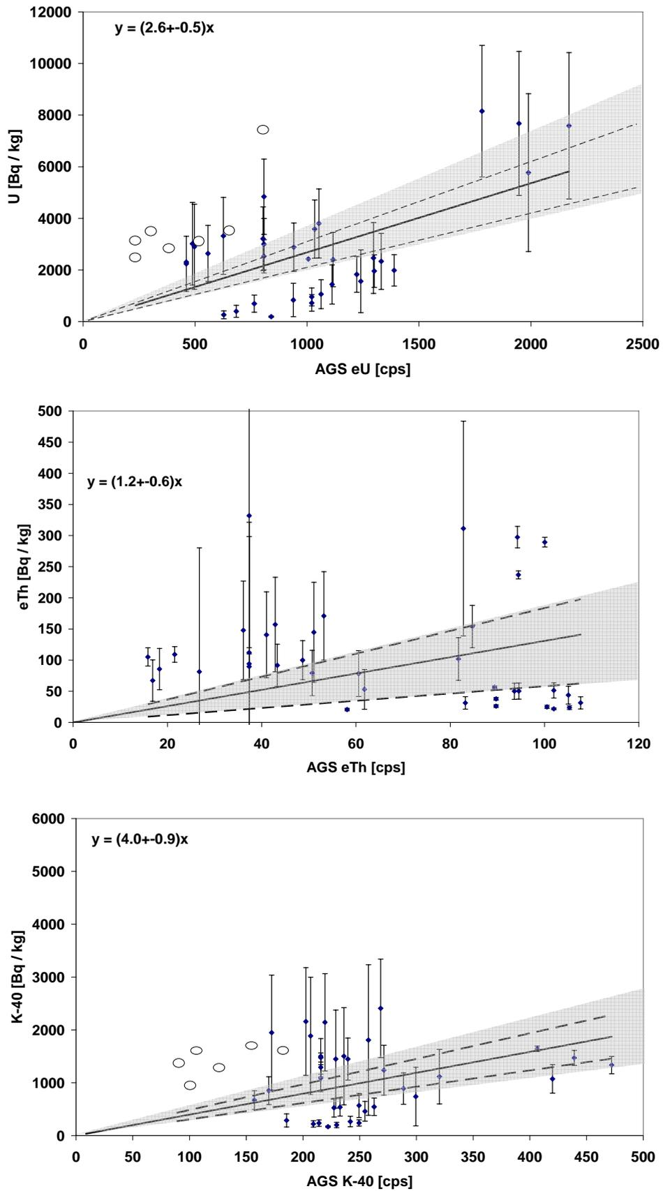
**Figure 19** Airborne versus ground measurements for eU, eTh and  $^{40}\text{K}$ . If positive outliers (3-sigma indicated by the shaded area) from the ground survey were rejected they are indicated by open circles and the remaining data points were used to derive the slope (solid) and 95% confidence interval (dashed). Error bars show one standard deviation of the mean of the groundbased measurements.
