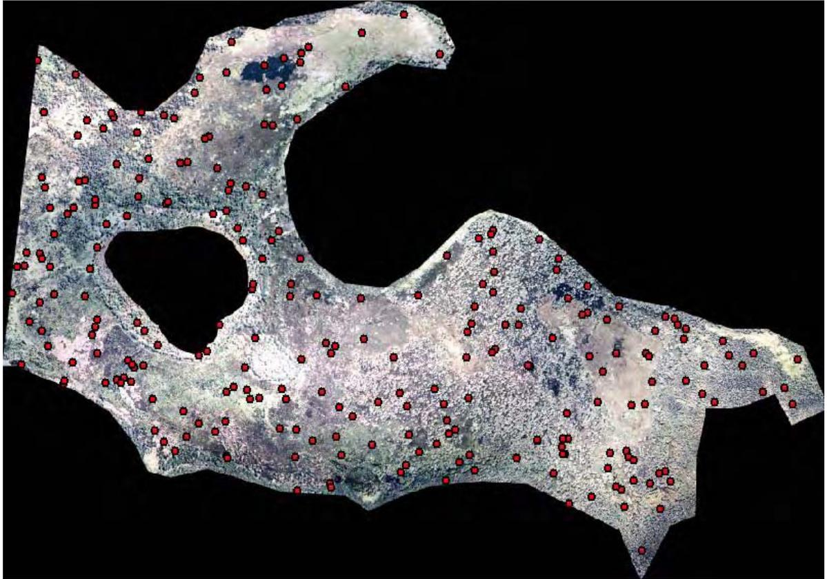
**Figure 3.5** Location of the 250 random points used to generate reference data for error assessment for the level 1 automated and final classified datasets
