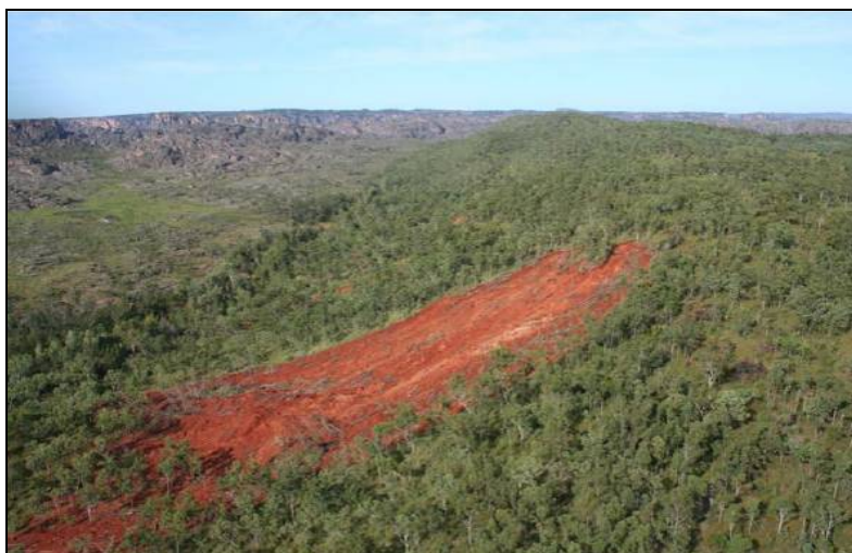
Figure 4 Landslip on weathered Oenpelli dolerite located in the upper catchment of Magela Creek (photo by Mike Saynor)
