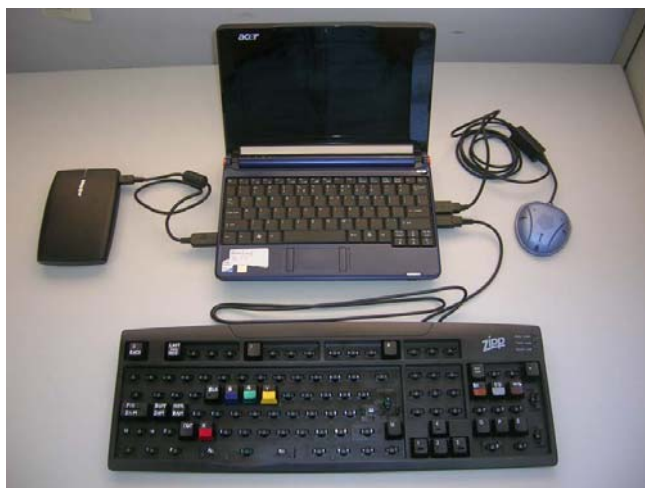
Figure 7 Layout of data recording system for aerial survey. A customised keyboard (unwanted keys removed) is connected to a small laptop with an in-built GPS recorder. Data is entered directly into the keyboard and downloaded following a survey session.
