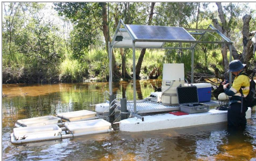
Figure 4 Picture of Magela Creek upstream (control) toxicity monitoring location showing test containers trailing from floating pontoon bearing water quality instrumentation
