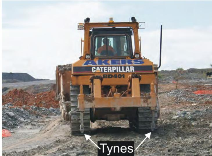
**Figure 2** Tynes on the back of a large bull dozer. The tynes are raised when not ripping the surface.
