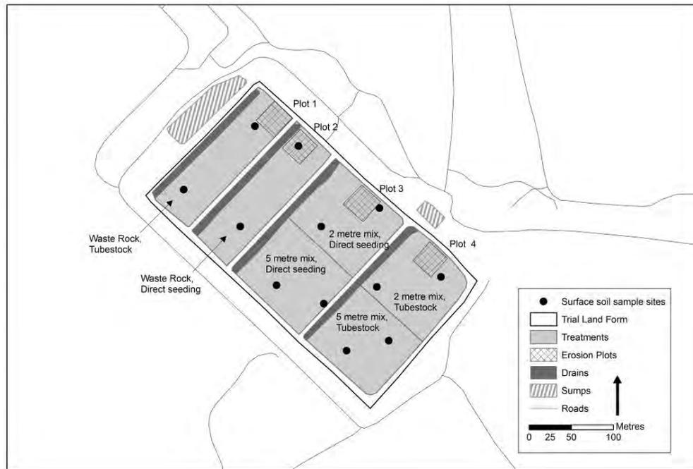
**Figure 4** Surface treatments and layout of erosion plots on the trial landform
