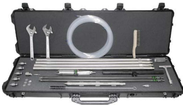
**Figure 7** AMS Piezometer Groundwater Sampling Kit. Includes stainless steel slotted section with four extensions, allowing samples to be collected to a depth of 3.6 m
