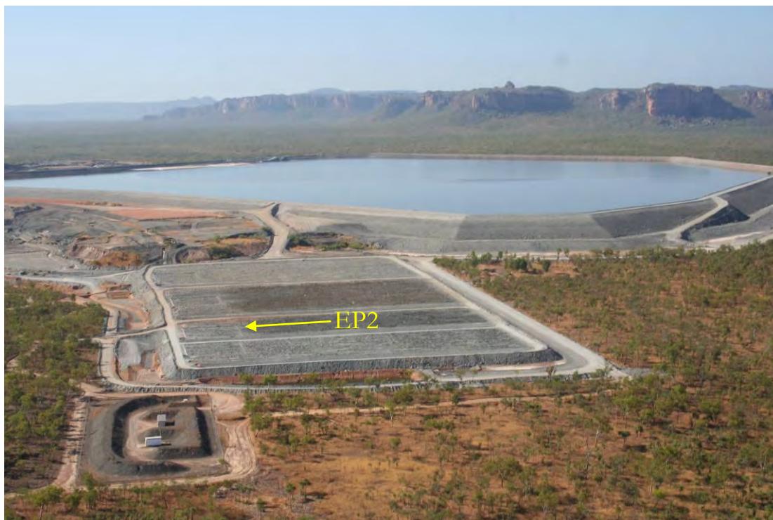
Figure 2 Aerial view of the completed trial landform located next to the Ranger mine Tailings Storage Facility (taken 28 August 2009)
