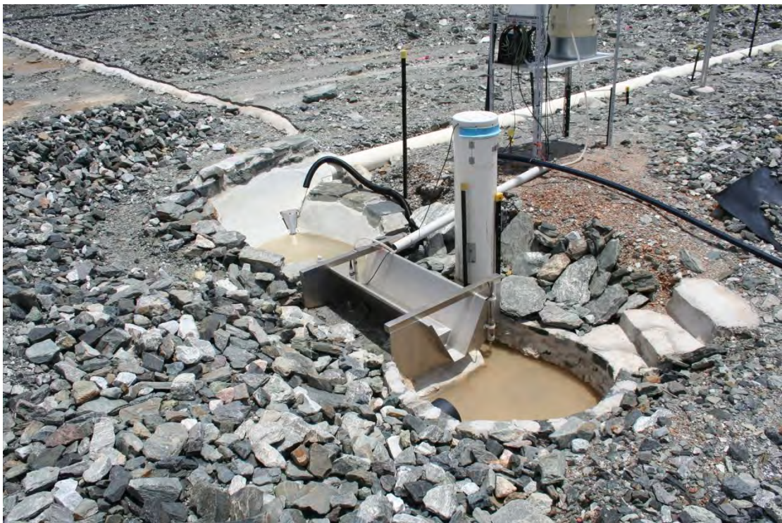
Figure 4 Flume, upstream stilling-basin and downstream draining-basin of EP2 (2 February 2010).
