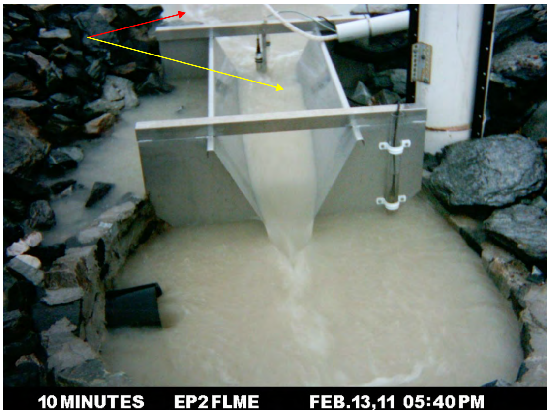
Figure 21 Water through EP2 flume at 5:40 pm on 13 February 2011. Although a poor field of view the disturbance in the upstream stilling basin can just be seen at the top of the image (red arrow) and the uneven flow through the flume is shown by the yellow arrow.
