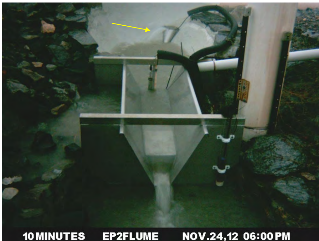
Figure 8 Flow through TLF2 flume at 6:00 pm, flow is starting to be deflected by the stainless cage, indicated by the yellow arrow.
