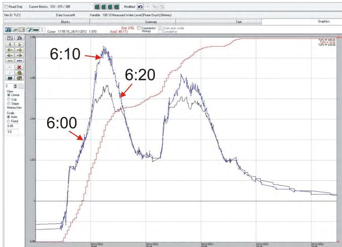
Figure 11 Example of the difference in water level between the stage trace and pressure transducer at higher runoff flows. The blue line (higher peaks) is the EP2 pressure transducer and black line is the shaft encoder. The red line is the cumulative rainfall for the event.
