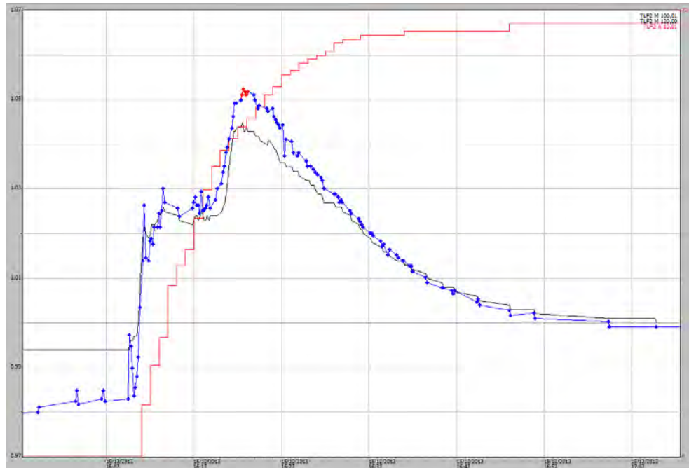
Figure A3- 24 Event 31 hydrograph from 15 December 2013. Blue is the pressure transducer and black is the shaft-encoder.
