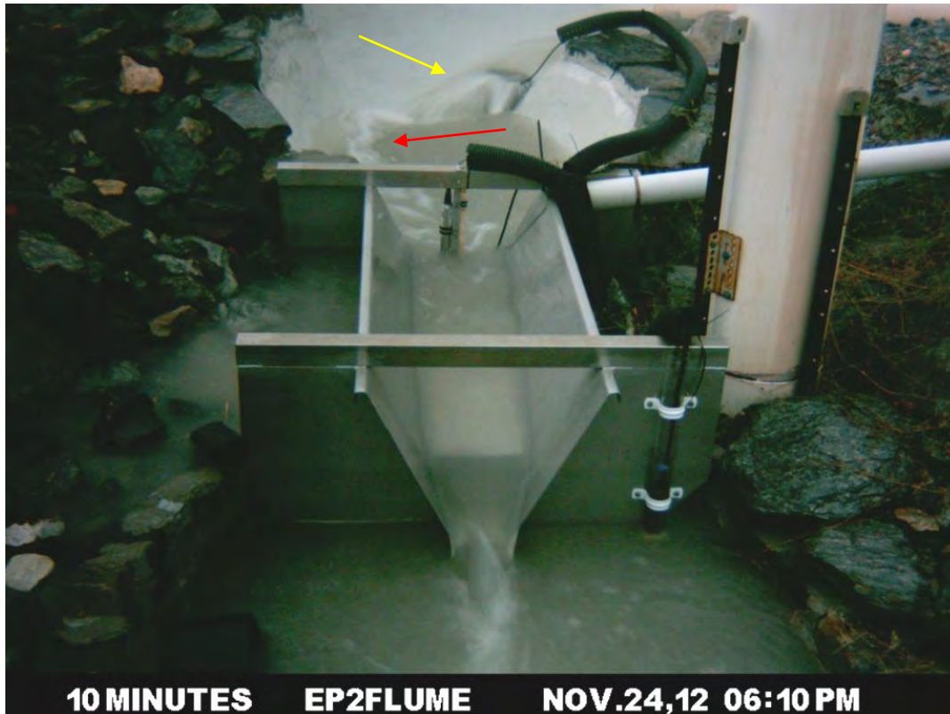
Figure 9 Flow through TLF2 flume at 6:10 pm, flow is being affected. The flow can be seen deflecting off the cage (yellow arrow) and can be seen rising up around the outside of the basin (red arrow).
