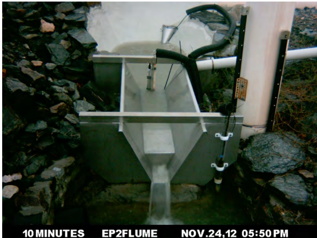
Figure 7 Flow through TLF2 flume at 5:50pm, uniform steady flow.
