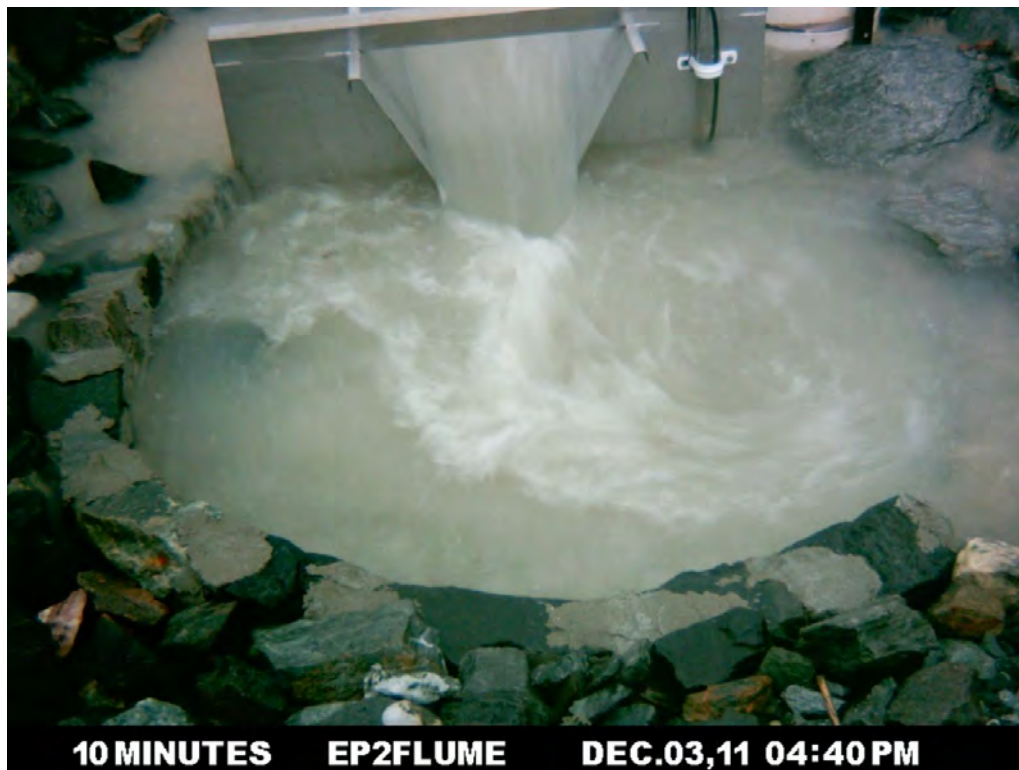
Figure 26 Flow through the flume on EP2 at 4:40 pm (time of the highest flow). The upstream basin cannot be seen in the image.
