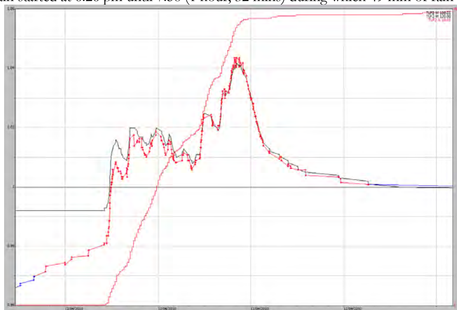
Figure A3-3 Event 4 hydrograph on 9 April 2010 both the pressure transducer (red) and the shaft-encoder (black) stage traces are very similar. 0.895m has been added to the pressure transducer.
