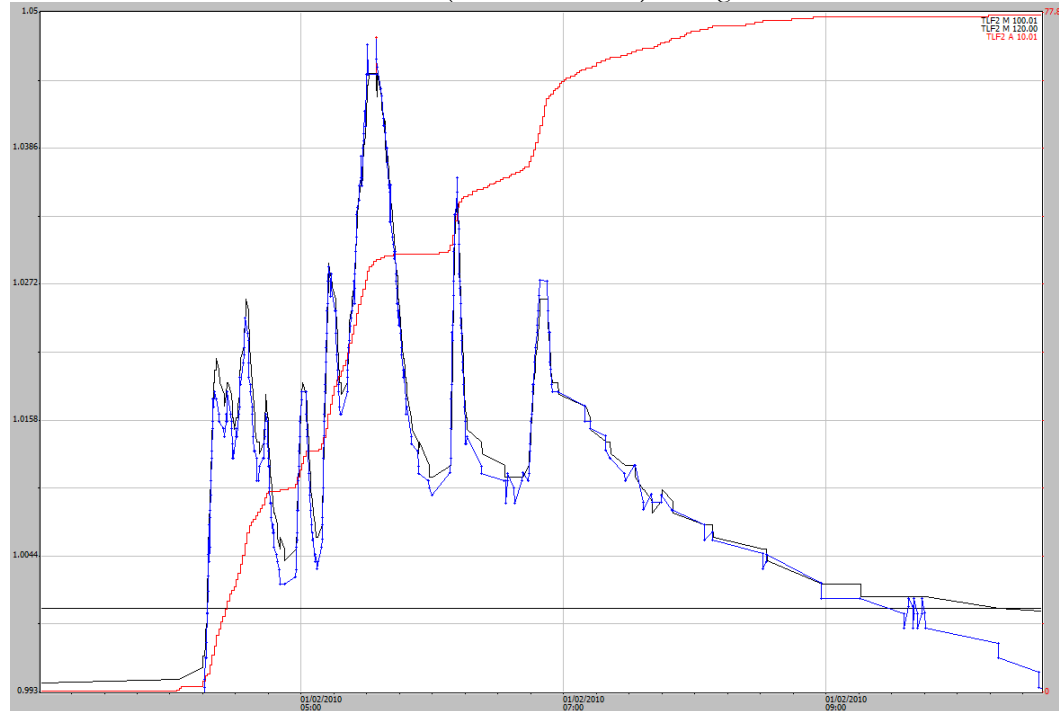
Figure A3-1 Event 2 hydrograph on 1 February 2010 both the pressure transducer (blue) and the shaft-encoder (black) stage traces are very similar. 0.895m has been added to the pressure transducer.
