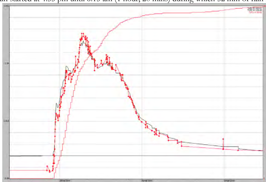
Figure A3-2 Event 3 hydrograph on 9 April 2010 both the pressure transducer (red) and the shaft-encoder (black) stage traces are very similar. 0.894m has been added to the pressure transducer.
