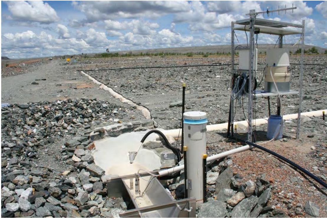
Figure 3 Across EP2, showing the upstream stilling-basin, part of the flume and the shelter for the data logger (2 February 2010).
